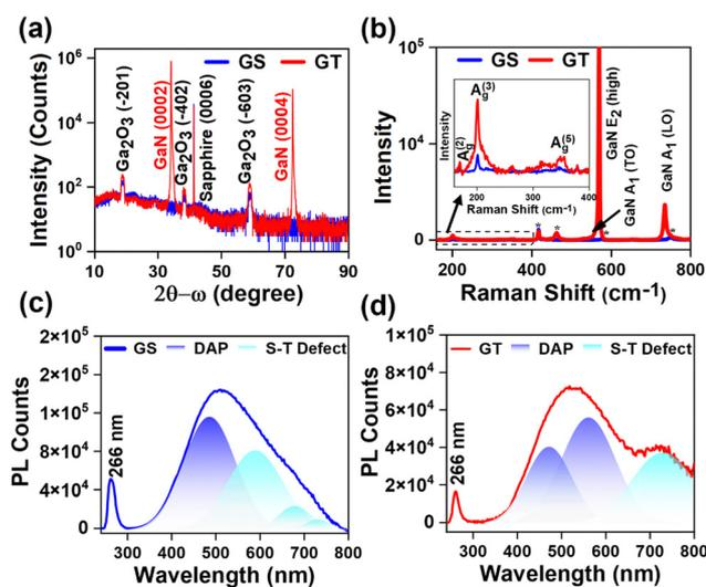
Fig. 1 (a) HRXRD  $2\theta - \omega$  scan and (b) Raman spectra of the GS (Ga<sub>2</sub>O<sub>3</sub>/sapphire) and GT (Ga<sub>2</sub>O<sub>3</sub>/p-GaN/sapphire) samples. (c) and (d) Fitted PL spectra of the GS and GT samples, respectively.
