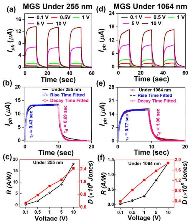
Fig. 5 The MGS device's (a) transient ( $I-t$ ) photo response curve, (b) fitted time response curve, and (c) the responsivity and detectivity versus voltage graph of MGS under 255 nm illumination. The (d) transient ( $I-t$ ) photo response curve, (e) fitted time response curve, and (f) the responsivity and detectivity versus voltage graph of MGS under 1064 nm illumination.
