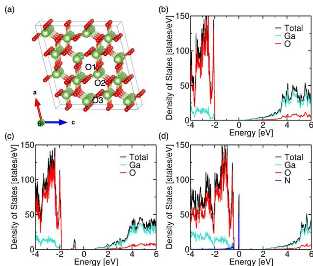
Fig. 3 (a) Crystal structure of  $\text{Ga}_2\text{O}_3$ . Atom projected partial density of states of (b) pristine, (c) O-vacant (O-vacancy at the O3-site), and (d) N-substituted  $\text{Ga}_2\text{O}_3$  (N-substitution at the O3-site).
