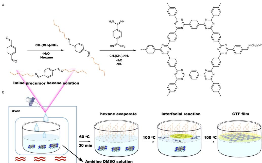
Fig. 25 Interfacial polymerisation of the CTF-HUST-film by Hu *et al.* Reprinted under CC-BY 4.0 License.<sup>180</sup>
