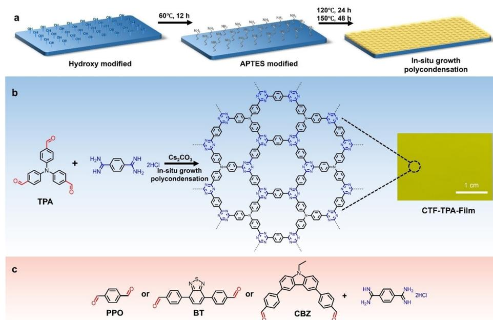
Fig. 26 (a) Reaction steps of self-assembly monolayer to continuous CTF films. (b) The condensation reaction for CTF-TPA-Film, and optical picture of continuous CTF-TPA-Film grown on glass slide. (c) Monomer building blocks used in the study. Figure adapted from ref. 181 Copyright 2023, Wiley-VCH GmbH.
