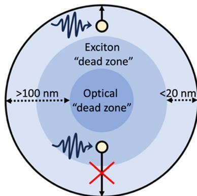
Fig. 4 Schematic example of a particulate photocatalyst depicting: photoexcitation and exciton migration, the exciton “dead zone”, and the optical “dead zone”.<sup>10,60</sup>
