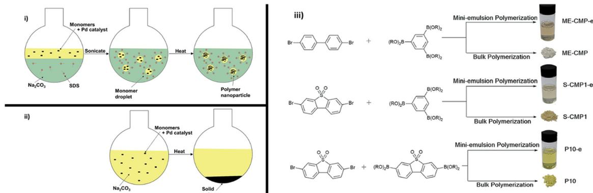
Fig. 13 Mini-emulsion polymerisation utilised by Aitchison *et al.* Reproduced under CC-BY 3.0 License.<sup>113</sup>
