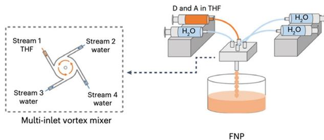
Fig. 11 Schematic representation of the flash nanoprecipitation method utilised by Yu *et al.* to prepare PNPs and nanofibers. Adapted under CC-BY 4.0 License.<sup>123</sup>
