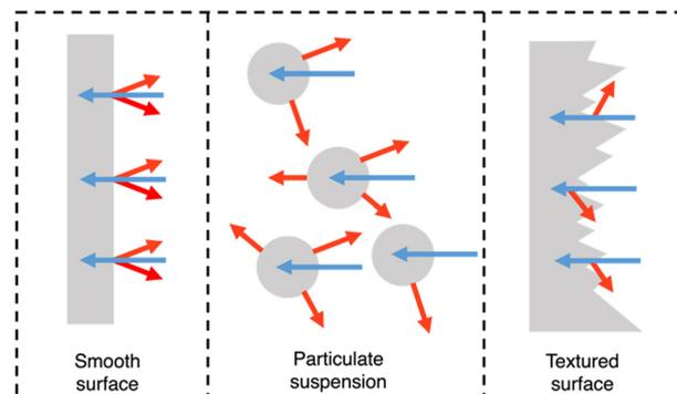
Fig. 18 Light distribution in flat and nanostructured films, and in particle suspensions. Blue arrows signify incident light and red arrows signify scattered/reflected light. *N.B.* the size of the arrows do not signify intensity of light scattering.<sup>164</sup>
