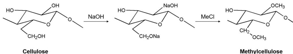
Fig. 8 The mechanism of methylcellulose synthesis.<sup>162</sup>
