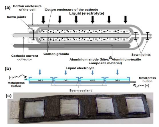
Fig. 7 (a) Schematic design of a textile-based flexible AAB. Side view (b) and the actual photograph (c) of the multi-cell battery with cells arranged on a plane. Reproduced from ref. 43 with permission from [Springer Nature], copyright [2021].
