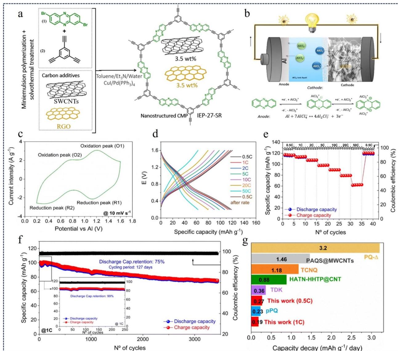
Fig. 15 (a) Synthesis strategy for IEP-27-SR mixtures. (b) Scheme of the aluminium–phenazine battery. (c) CV recorded at  $10 \text{ mV s}^{-1}$ . (d) GCD profiles of the Al//IEP-27-SR battery. (e) Battery rate performance. (f) Long-term cycle stability of an Al//IEP-27-SR battery. (g) Capacity fade per day.<sup>107</sup> Copyright 2023, Royal Society of Chemistry.
