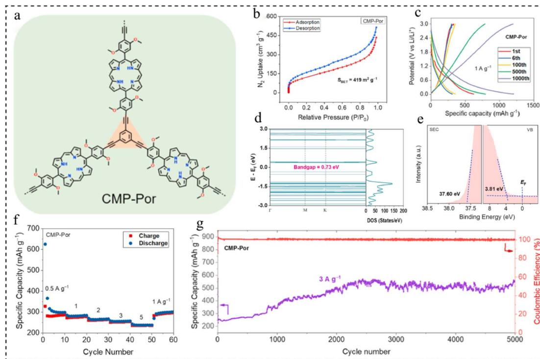
Fig. 12 (a) Structure of CMP-Por. (b) BET test for CMP-Por. (c) GCD profiles at  $1 \text{ A g}^{-1}$ . (d) Density of states of CMP-Por. (e) Ultraviolet photoelectron spectroscopy of CMP-Por. (f) Rate capability. (g) Long-term cycle life at  $3 \text{ A g}^{-1}$ .<sup>103</sup> Copyright 2022, Elsevier.
