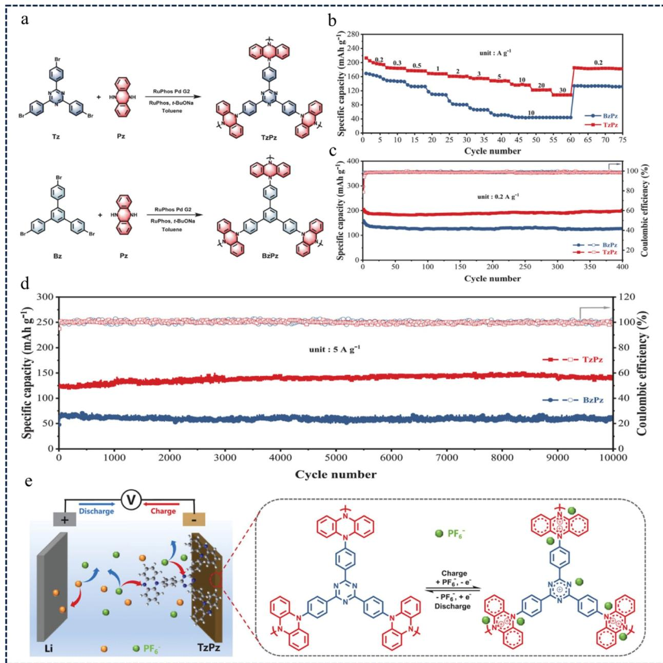
Fig. 16 (a) The synthetic reaction route of TzPz and BzPz. (b) The rate performance at current densities from 0.2 to 30 A g<sup>-1</sup>. (c) Cycling performance at current densities of 0.2 A g<sup>-1</sup> and (d) 5 A g<sup>-1</sup>. (e) Schematic diagram of the electrochemical reaction mechanism of the TzPz-based cathode.<sup>112</sup> Copyright 2021, Wiley.
