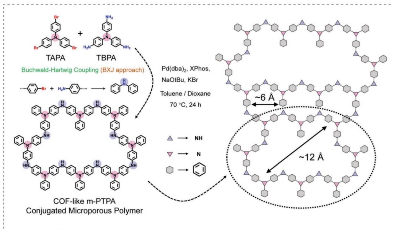
Fig. 14 The synthesis route of COF-like m-PTPA.<sup>106</sup> Copyright 2021, Wiley.
