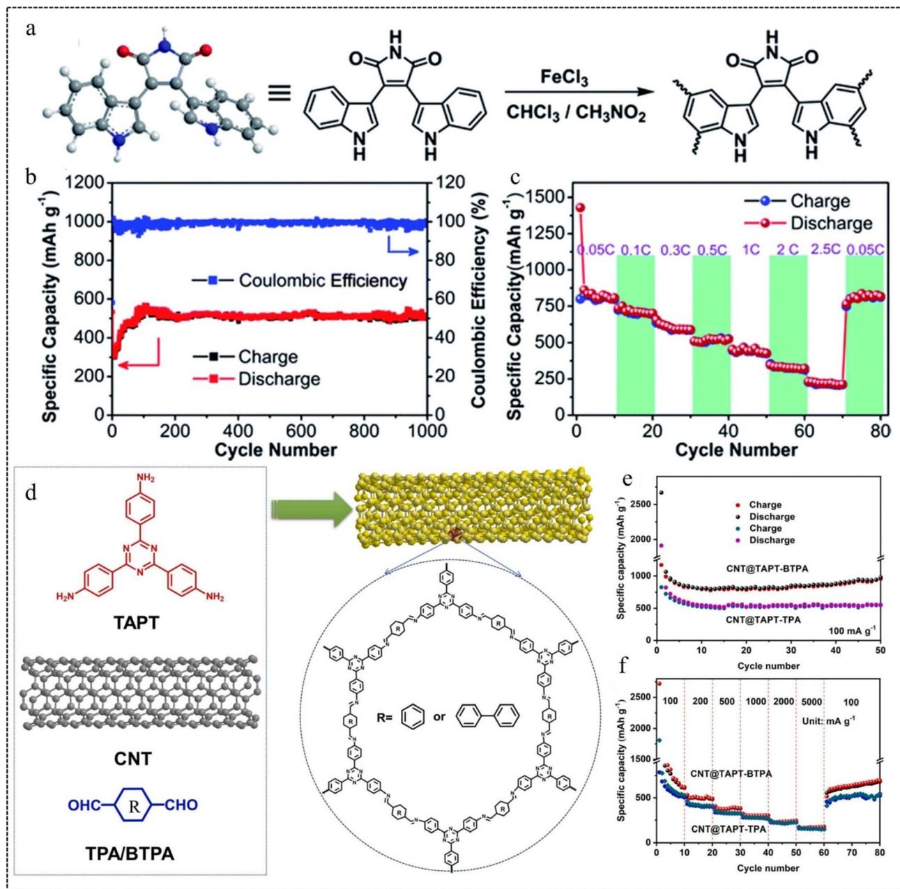
Fig. 6 Oxidative coupling polymerization routes. (a) Synthesis of PBIM. (b) Cycle performance of CMP-PBIM. (c) The rate performance at different current densities from 0.05C to 2.5C.<sup>67</sup> Copyright 2018, Royal Society of Chemistry. Schiff-base reaction routes. (d) Synthetic route of CNT@TAPT-TPA/BTPA. (e) Cycling performance of CNT@TAPT-TPA and CNT@TAPT-BTPA. (f) Rate performance of CNT@TAPT-TPA and CNT@TAPT-BTPA.<sup>68</sup> Copyright 2023, Elsevier.
