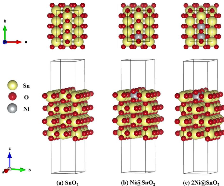
Fig. 1 Top and side view of chosen  $\text{SnO}_2(110)$  model systems for (a) bare  $\text{SnO}_2$ , (b) single Ni-doped  $\text{SnO}_2$  ( $\text{Ni@SnO}_2$ ), and (c) double Ni-doped  $\text{SnO}_2$  ( $2\text{Ni@SnO}_2$ ) systems.
