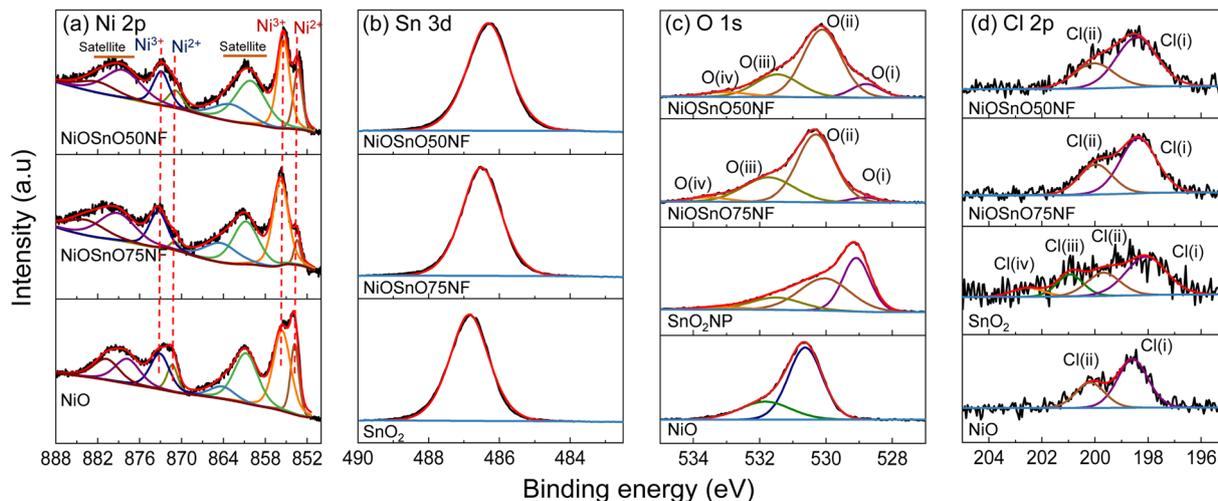
Fig. 4 (a) Ni 2p, (b) Sn 3d, (c) O 1s, and (d) Cl 2p XPS core spectra for NiOSnO50NF, NiOSnO75NF, NiO, and SnO<sub>2</sub>.
