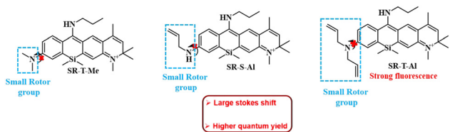
Fig. 13 Molecular structures of Si-Rhodamine-based probes containing small molecular rotor moieties. 99 [Open access].
