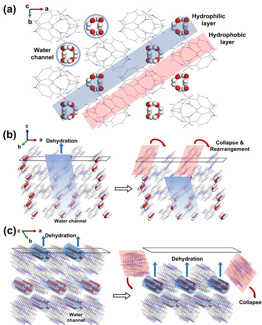
Fig. 5 (a) Supercell structures along the *c*-axis of crystals E1 and E2. Schematic diagrams of dehydration channel changes during the dehydration process (b) on E1 crystal face (0 0 1) and (c) on E2 crystal face (1 0 0).
