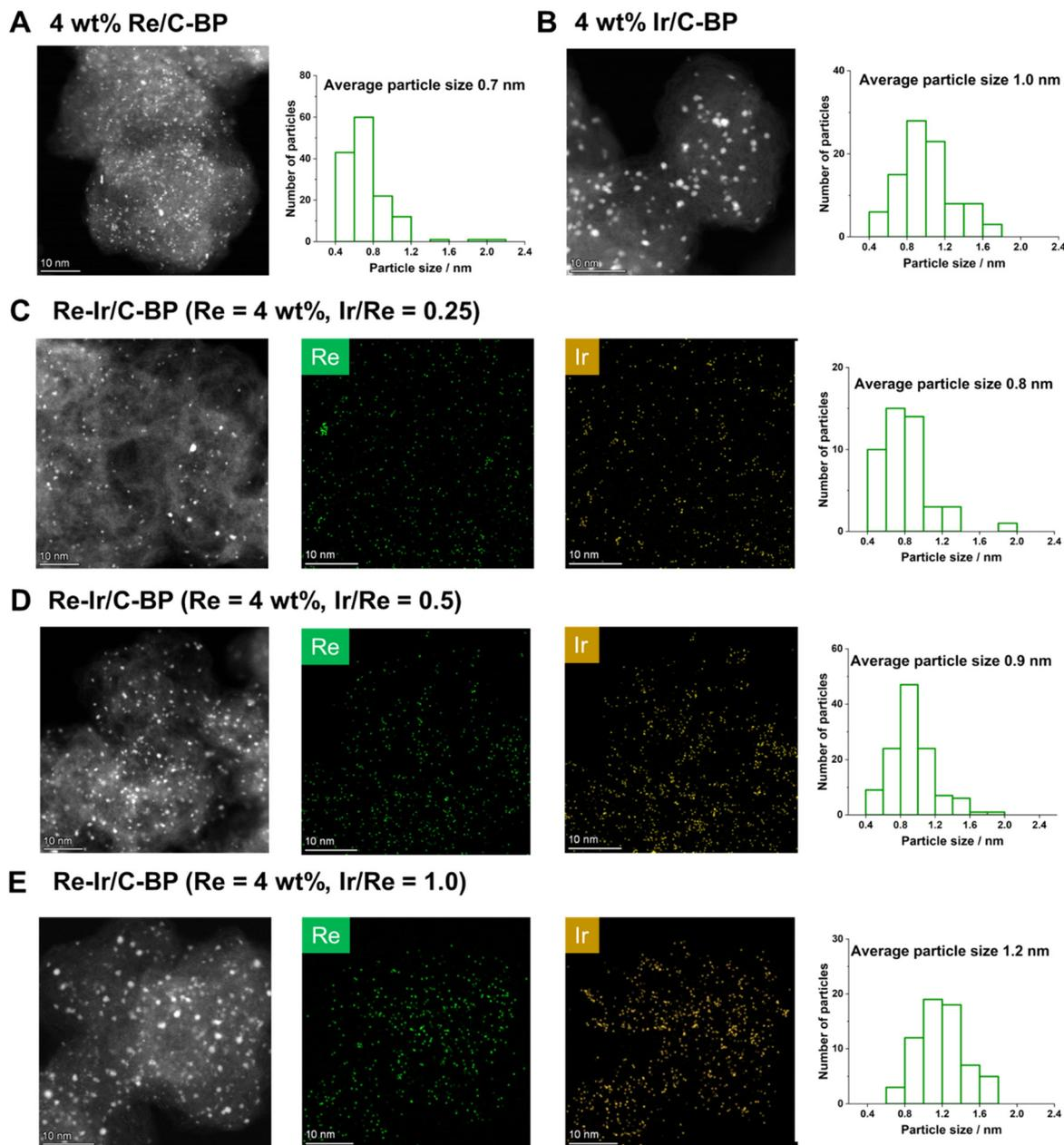
**Fig. 6** HAADF-STEM images and elemental mapping of catalysts after reduction ( $H_2$ , 773 K) + passivation: (A) Re/C-BP (Re 4 wt%); (B) Ir/C-BP (Ir 4 wt%); (C) Re-Ir/C-BP (Re 4 wt%, Ir/Re = 0.25); (D) Re-Ir/C-BP (Re 4 wt%, Ir/Re = 0.5); (E) Re-Ir/C-BP (Re 4 wt%, Ir/Re = 1.0).
