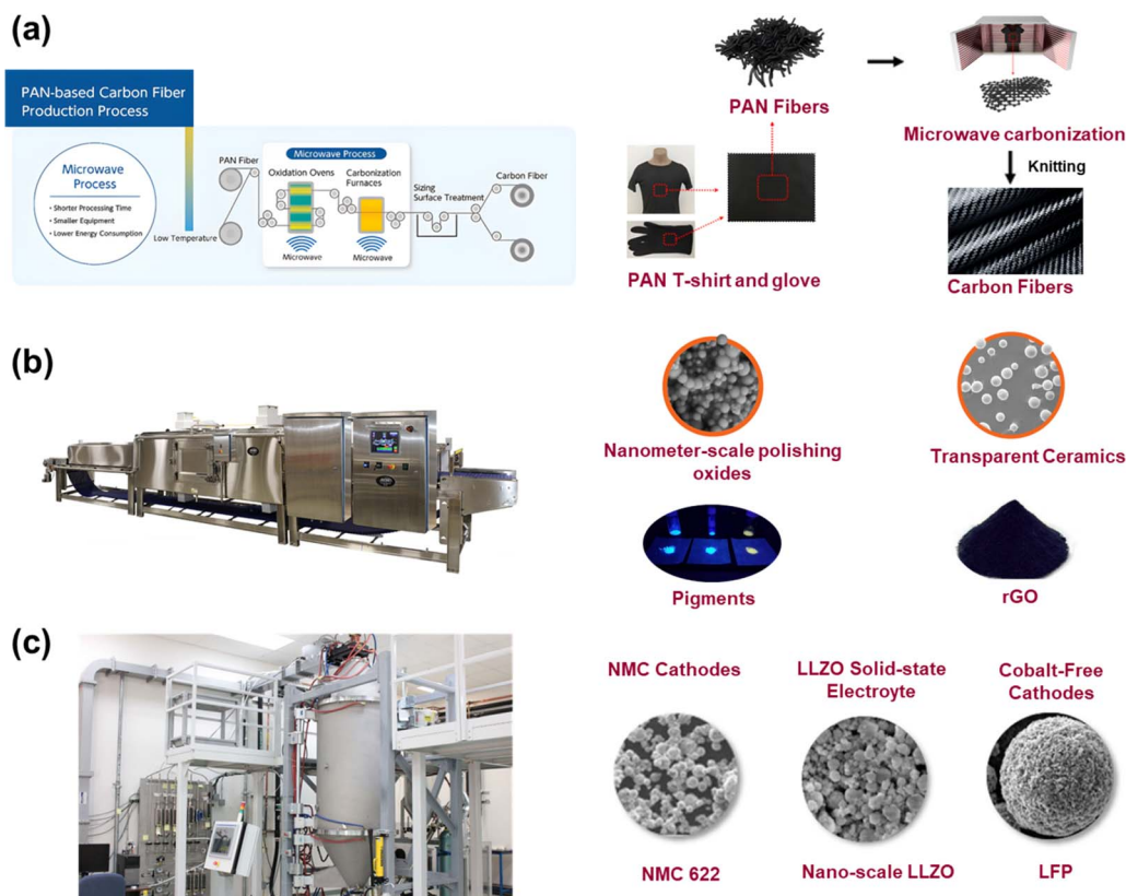
Fig. 5 (a) Schematic diagram of the microwave reactor for the production of carbon fibres and its applied products. (b) The UniMelt system of 6K Inc. and its applied products. (c) The microwave continuous processing reactor of AMTek and its applied products.
