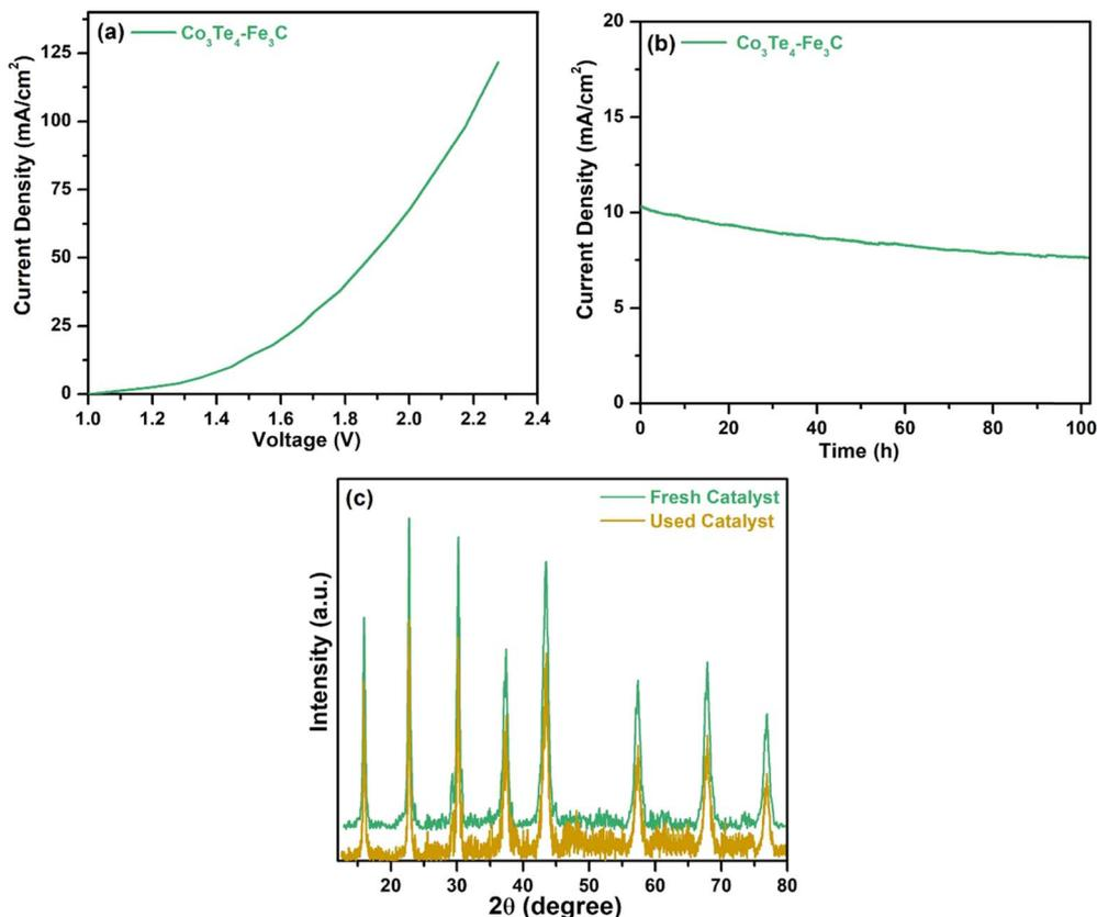
Fig. 7 (a) LSV polarization curve for overall water splitting, (b) chronoamperometric curve of  $\text{Co}_3\text{Te}_4\text{-Fe}_3\text{C}$  using an overall two electrode set-up, and (c) XRD pattern of the used catalyst after overall water-splitting.
