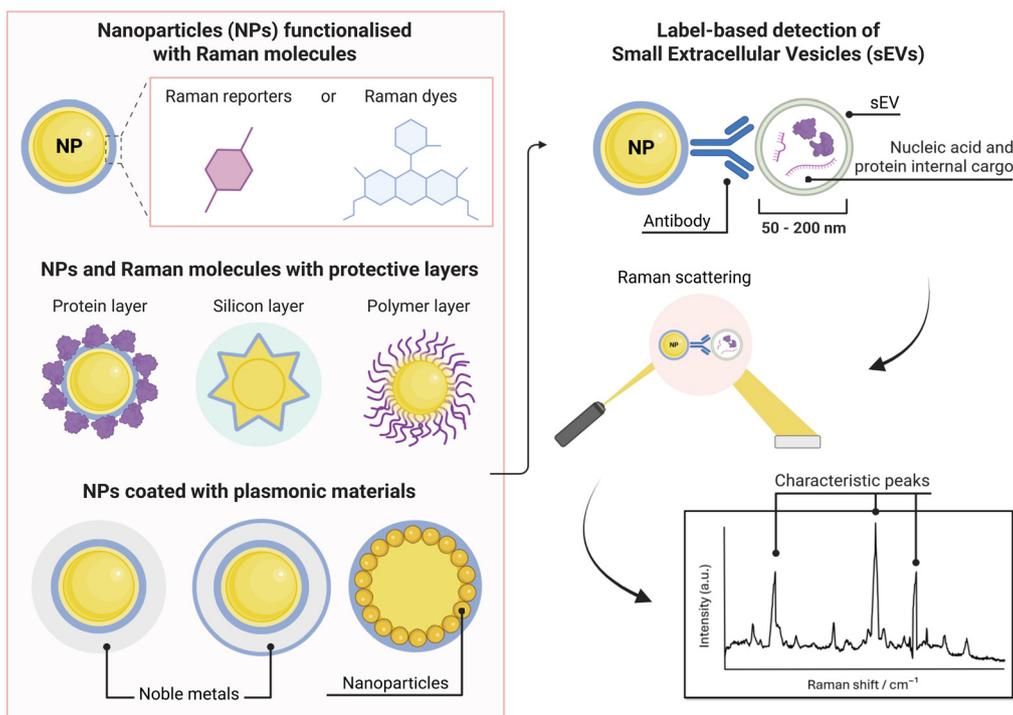
**Fig. 6** SERS nanotags for use in label-based assay designs including nanoparticle functionalization, protective layers, and coatings. And a scheme of the functionalized nanoparticle-sEV complex and corresponding characteristic peaks.
