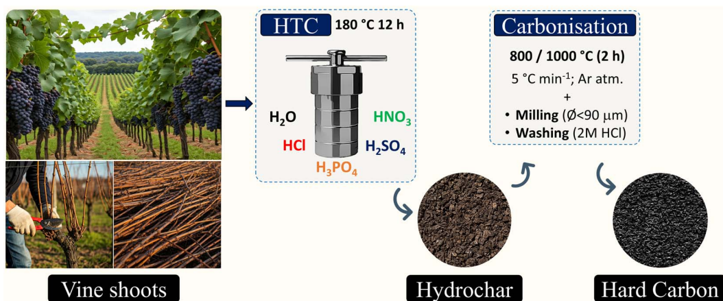
Fig. 1 Graphical summary of the hard carbon synthesis via HTC.
