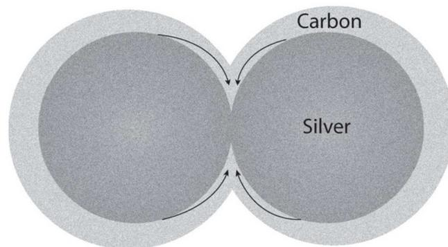
Figure 4: Sintering of two nanoparticles covered with a carbon surface coating, showing that for the neck to grow, atomic diffusion from the surface to the neck occurs through the carbon.
