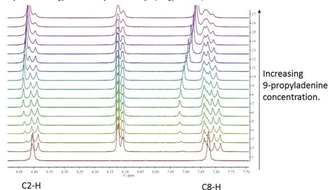
**Figure 3.** <sup>1</sup>H NMR spectrum illustrating shifts in the C8-H and C2-H proton signals during titration of mono-TP with 9-propyladenine. Spectrum 1 corresponds to pure 9-propyladenine and spectra 2-17 are recorded with constant mono-TP concentration and increasing 9-propyladenine concentration.
