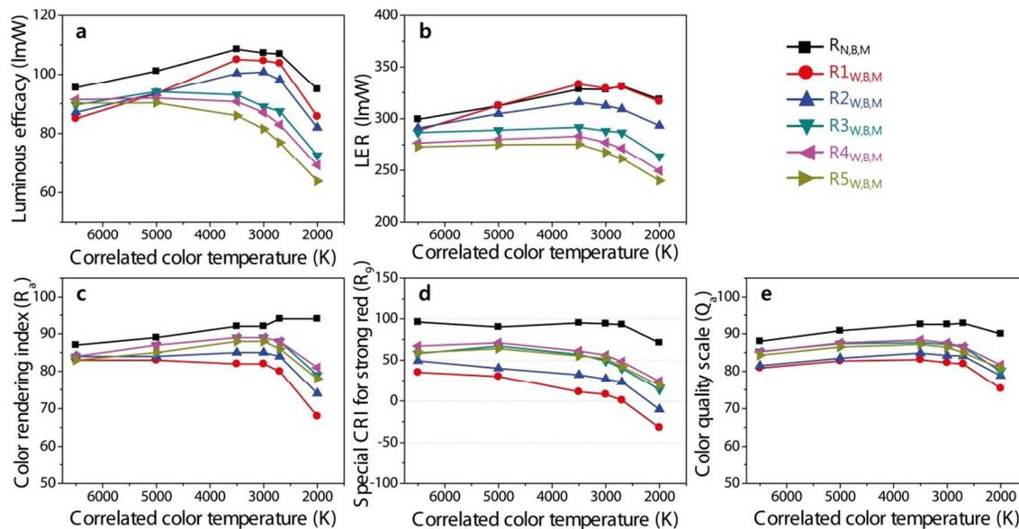
**Fig. 6.** The optical properties of the six combinations of four-package  $R_{B,M}A_{B,M}G_{B,M}B$  white LEDs at different CCTs with the various red phosphors: (a) LE, (b) LER, (c) CRI, (d)  $R_9$ , and (e) CQS.
