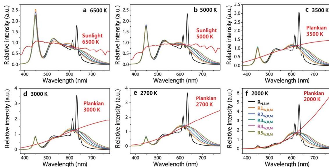
**Fig. 5.** The EL spectra of the six combinations of four-package  $R_{B,M}A_{B,M}G_{B,M}B$  white LEDs at different CCTs with the various red phosphors and the reference ideal (Planckian) or natural (sunlight) light sources of CRI at different CCTs: (a) 6500 K, (b) 5000 K, (c) 3500 K, (d) 3000 K, (e) 2700 K, and (f) 2000 K.
