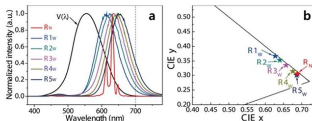
Fig. 2. (a) The photopic luminosity function (V(λ)) and normalized PL spectra of six red phosphors and (b) the 1931 color coordinates of the six red phosphors.
