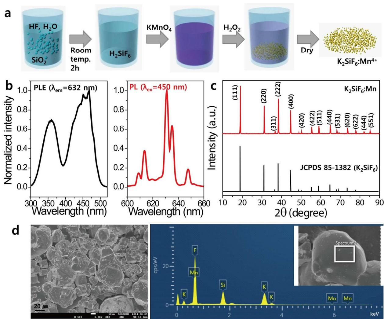
**Fig. 1.** (a) Schematic diagram of synthetic method of  $K_2SiF_6:Mn^{4+}$ , (b) the excitation and emission spectra, (c) powder XRD (JCPDS 85-1382 ( $K_2SiF_6$ )), and (d) FE-SEM and EDS data of the as-synthesized  $K_2SiF_6:Mn^{4+}$  phosphor.
