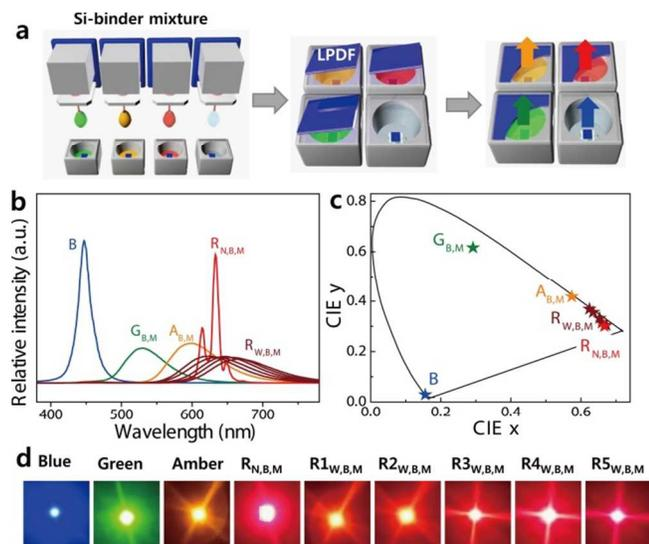
**Fig. 3.** (a) Schematic diagram of four-package white LED, (b) The EL spectra, (c) 1931 CIE color coordinates, and (d) photographs of the blue semiconductor-type LED and eight different colors of fully down-converted LPDF-capped pc-LEDs ( $G_{B,M}$ ,  $A_{B,M}$ ,  $R_{N,B,M}$ ,  $R1_{W,B,M}$ ,  $R2_{W,B,M}$ ,  $R3_{W,B,M}$ ,  $R4_{W,B,M}$ , and  $R5_{W,B,M}$ ).
