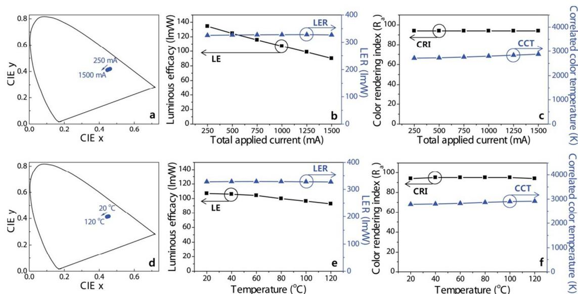
**Fig. 7.** Current dependence of the  $R_{N,B,M}A_{B,M}G_{B,M}B$  white LED at 2700 K at room temperature: (a) 1931 CIE color coordinates, (b) LE and LER, and (c) CRI and CCT. The temperature dependence of the  $R_{N,B,M}A_{B,M}G_{B,M}B$  white LED at 2700 K with a total applied current of 1000 mA: (d) 1931 CIE color coordinates, (e) LE and LER, and (f) CRI and CCT.
