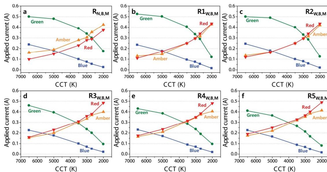
**Fig. 4.** The fractional applied currents of the primary LEDs in six combinations of four-package  $R_{B,M}A_{B,M}G_{B,M}B$  white LED at different CCTs with the various red phosphors: (a)  $R_{N,B,M}$ , (b)  $R1_{W,B,M}$ , (c)  $R2_{W,B,M}$ , (d)  $R3_{W,B,M}$ , (e)  $R4_{W,B,M}$ , and (f)  $R5_{W,B,M}$ .
