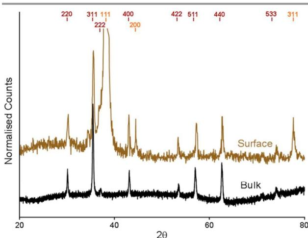
**Fig. 4** XRD data recorded for the MNPs biomineralised by Mms6 onto gold (gold) and of the control particles that form in solution (black) during a POFHK reaction. The expected peak positions for magnetite (red) and gold (gold) are highlighted.
