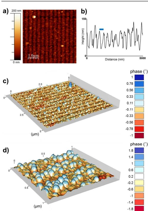
**Fig. 3** Tapping mode AFM image (a), an example height profile across a section of the tapping mode AFM image (b) and composite images of tapping mode AFM and MFM phase shift at a lift height of 50 nm (c and d, scales in  $\mu\text{m}$ ) of a MNP array biotemplated by Mms6 after patterning by IL. Blue bar represents the average period (357 nm).
