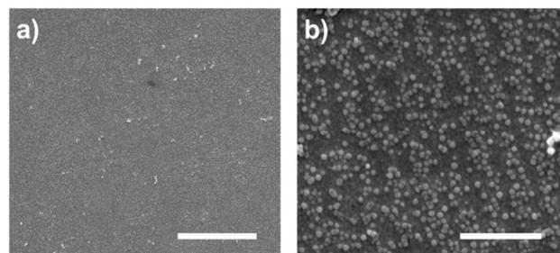
**Fig. 5** SEM images of gold surfaces covered with a complete layer of cysteine-tagged Mms6 protein that were patterned by IL at an exposure dose of  $100 \text{ J cm}^{-2}$ , after backfilling with OEG-thiolate and being subjected to a POHFK reaction. Scale bars: a –  $10 \mu\text{m}$  and b –  $1 \mu\text{m}$ .
