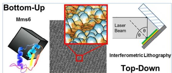
Top-down surface patterning technique, interferometric lithography, is combined with bottom-up magnetite nanoparticle biomineralisation using Mms6 to form magnetic nanoscale arrays.
