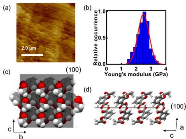
**Figure 1** AFM and X-ray data for macro-sized aspirin (form I): (a) AFM height image of (100) face of macro-dimensional crystal, (b) histogram of Young's moduli for both (100) and (-100) planes (Gaussian fit in red), (c) packing along (100) planes showing exposed acetyl groups in space-fill, and (d) hydrogen-bonded dimers of the (100) face (CSD refcode: ACSALA01).<sup>18</sup>
