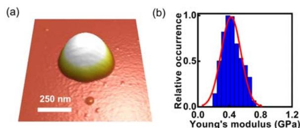
**Figure 2** AFM data for nano-sized aspirin (Form I): (a) representative AFM height image and (b) histogram of Young's moduli data obtained on 12 different nanocrystals (Gaussian fit in red).
