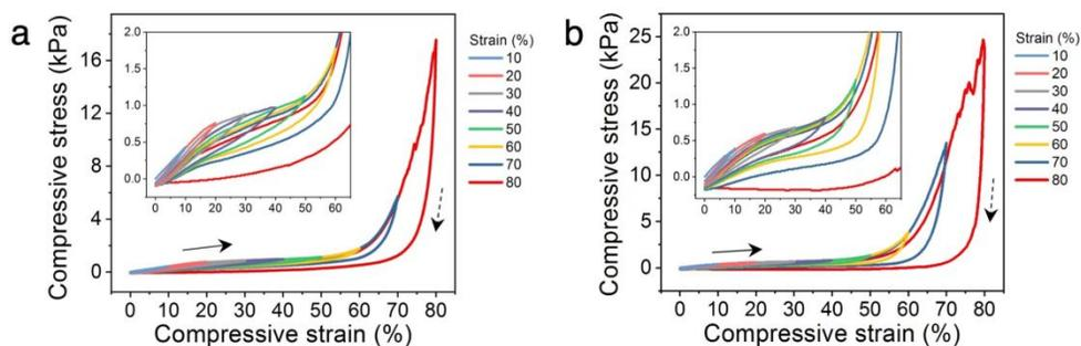
**Figure 5.** Cyclic compression behavior of PANI hydrogels. Stress-strain curves during loading-unloading to various strains for (a) Kelvin lattice with 14% relative density, and (b) octet lattice with 16% relative density. Arrows and dashed arrows represent the loading and unloading directions, respectively. A loading and unloading rate of  $100\% \text{ min}^{-1}$  was used.
