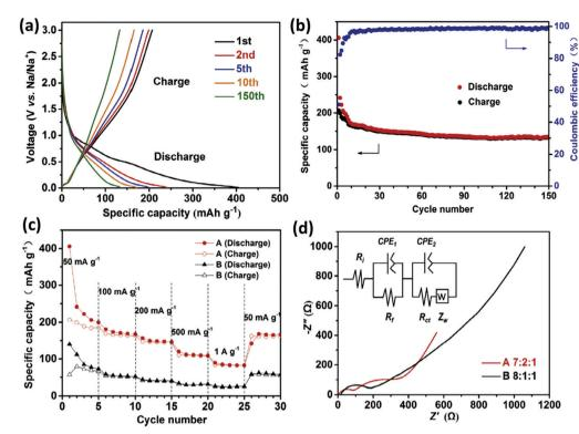
**Fig. 8** Electrochemical performance corresponding to  $MgFe_2O_4$  micro-box electrodes with varying ratios of the active material, *viz.*, A (7:2:1) and B (8:1:1). (a) Discharge-charge potential profiles and (b) cyclic stability performance at 50 mA g<sup>-1</sup> of sample A; (c) rate capability and (d) Nyquist plots corresponding to samples A and B. Reprinted with permission from ref. 9. Copyright 2017 Elsevier.
