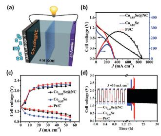
**Fig. 14** Electrochemical performance of the  $Co_{0.85}$ Se@NC cathode incorporated Zn-air battery: (a) Schematic representation of rechargeable Zn-air battery. (b) Polarization plot (*V*-*i*) and associated power density plot. (c) Charge/discharge potential (*V*-*i*) plots. (d) Cyclic stability performance. Reprinted with permission.<sup>25</sup> Copyright 2017 Royal Society of Chemistry.
