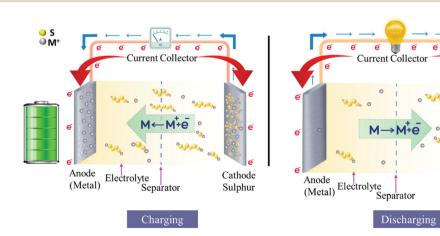
Fig. 4 Charging and discharging mechanism for an MS battery.
