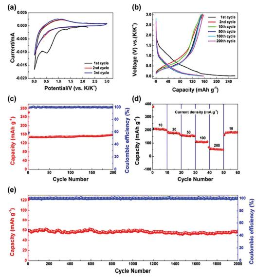
**Fig. 6** Electrochemical characteristics of MIL-125 (Ti) MOF as the anode for potassium-ion batteries. (a) Cyclic voltammetry (CV) loops at 0.5 mV s<sup>-1</sup>. (b) Galvanostatic charge–discharge plots at 50 mA g<sup>-1</sup>. (c) Cyclic stability was exhibited at 50 mA g<sup>-1</sup>. (d) Rate performance at various current densities. (e) Long-term cyclic stability at 200 mA g<sup>-1</sup>. Reprinted with permission from ref. 86. Copyright 2017 Royal Society of Chemistry.
