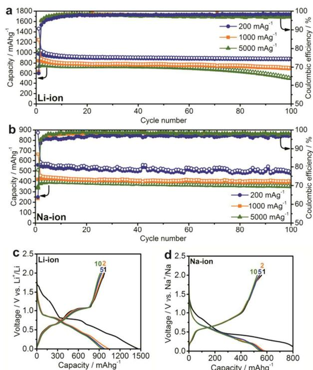
**Figure 2.** Electrochemical performance of SnSb NCs. Capacity retention for SnSb NCs in (a) Li-ion and (b) Na-ion half-cells at a current of 200, 1000 and 5000 mA g<sup>-1</sup>. Galvanostatic charge and discharge curves for SnSb NCs in (c) Li-ion and (d) Na-ion half-cells at a current of 200 mA g<sup>-1</sup>. All measurements were performed in the potential range of 0.005–2.0 V.
