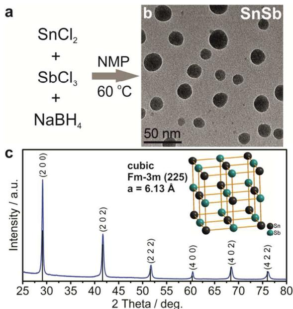
**Figure 1.** Synthesis and characterization of SnSb NCs. (a) Reaction scheme. (b) Transmission electron microscopy (TEM) image. (c) X-ray diffraction (XRD) pattern of SnSb NCs, indexed as cubic SnSb (COD entry 9008724).
