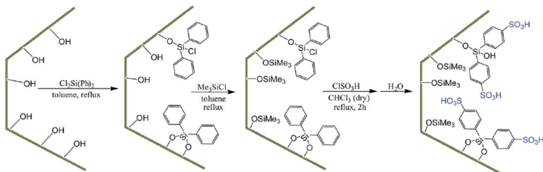
Fig. 36 Preparation of SBA-15-Ph-SO<sub>3</sub>H. Reprinted from ref. 158 with permission of Royal Society of Chemistry.
