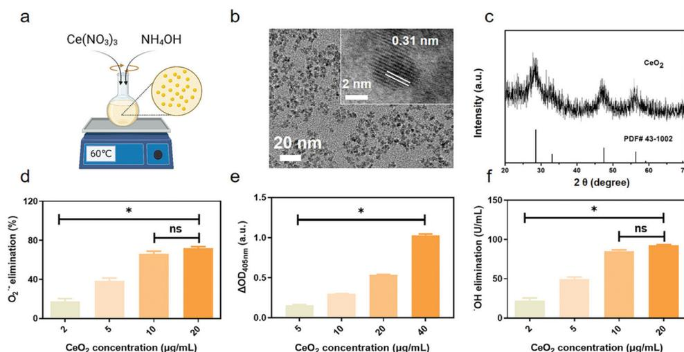
**Fig. 1** The characterization analysis and enzyme-mimicking activities of CeO<sub>2</sub> NPs. (a) Synthesis scheme of CeO<sub>2</sub>; (b) TEM images; (c) XRD spectrum; (d) SOD-like activity of CeO<sub>2</sub> NPs at different concentrations; (e) CAT-like activity; and (f) •OH elimination ability. ns means  $P > 0.05$  and \* means  $P < 0.05$ .
