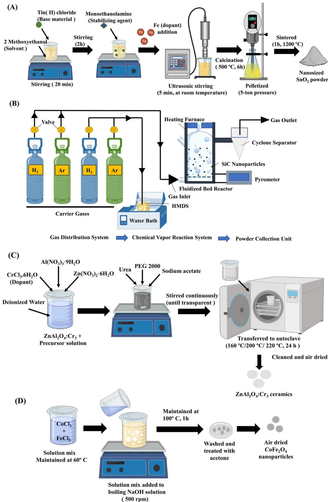
Fig. 3 Synthesis methods of nanobioceramics. (A) Schematic illustration of Fe-doped SnO<sub>2</sub> nanopowder prepared by the sol-gel technique.<sup>42</sup> (B) Synthesis of SiC nanoparticles by fluidized bed chemical vapor deposition method.<sup>43</sup> (C) Preparation of ZnAl<sub>2</sub>O<sub>4</sub>:Cr<sub>3</sub> ceramics by solvothermal method.<sup>45</sup> (D) Chemical precipitation of CoFe<sub>2</sub>O<sub>4</sub> nanoparticles.<sup>46</sup>
