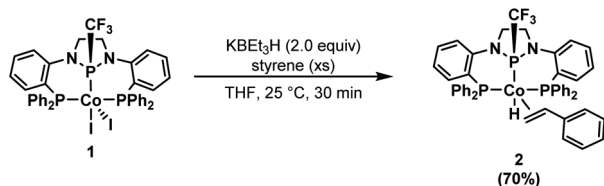
Scheme 2 Synthesis of (\text{PP}^{\text{CF}_3}\text{P})\text{Co}(\eta^2\text{-styrene})\text{H} ( 2 ), the primary metal-containing species observed spectroscopically during catalytic turnover.
