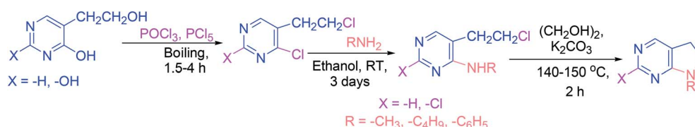
Scheme 19 Synthesis of 5,6-dihydropyrrolo[2,3- d ]pyrimidines.
