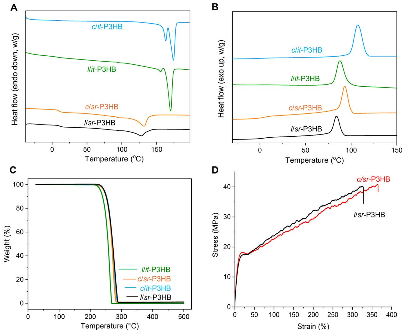
**Fig. 3** (A) Overlay of DSC trace, 2<sup>nd</sup> heating scan (10 °C min<sup>-1</sup>). (B) Overlay of DSC trace cooling scan (10 °C min<sup>-1</sup>). (C) Representative stress–strain curves of //sr-P3HB (black, 283 kg mol<sup>-1</sup>,  $\bar{D}$  = 1.26) and c/sr-P3HB (red, 163 kg mol<sup>-1</sup>,  $\bar{D}$  = 1.28). Strain rate = 5 mm min<sup>-1</sup>. (D) Decomposition temperature overlay of P3HB produced in this work.
