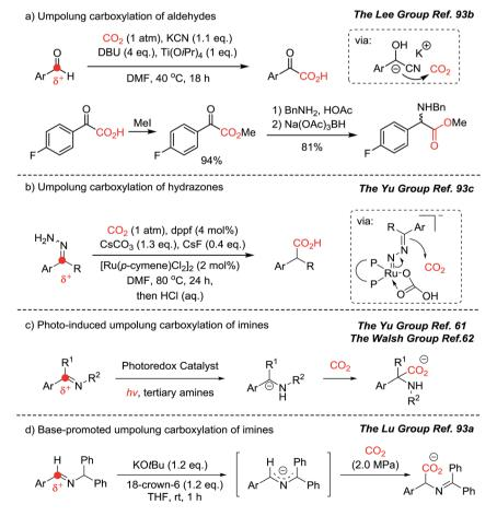
Scheme 23 Direct umpolung carboxylation. (a) Umpolung carboxylation of aldehyde and reductive amination of  $\alpha$ -keto acids to  $\alpha$ -amino acids; (b) umpolung carboxylation of hydrazones; (c) photo-induced and (d) base-promoted umpolung carboxylation of imines.
