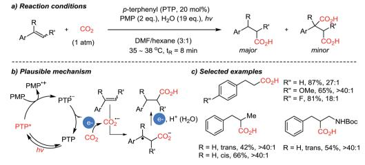
Scheme 10 Photocatalytic direct β-selective hydrocarboxylation of styrenes.
