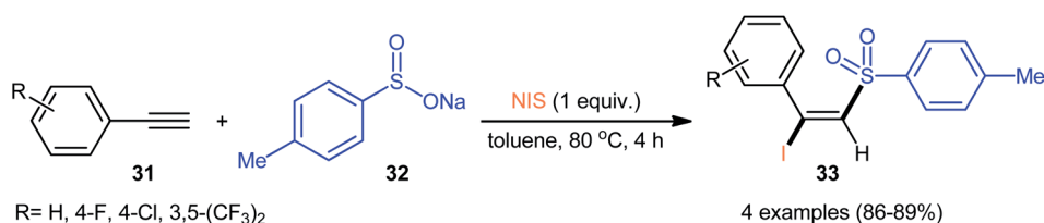
Scheme 14 Catalyst-free iodosulfonylation of terminal aromatic alkynes 31 with sodium p -toluenesulfonate 32 and NIS.
