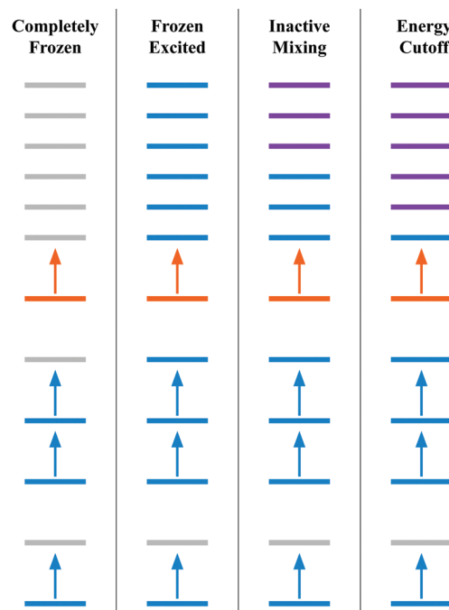
Fig. 1 A general scheme showing the approximations used in the optimization strategies employed on \text{SF}_6 . The diagrams do not exactly represent \text{SF}_6 because many more electrons and orbitals are required. Each section represents a determinant diagram where the colors are used to show in which subspace the basis function and electron reside. Here, blue represents the core electrons subspace, orange represents the excited electron subspace, purple represents being in both the core electron and excited electron subspaces, and gray represents being excluded entirely. Each line represents a reference orbital ( i.e. the ground state molecular orbitals), and the arrows represent electron occupation at the start of the calculations.
