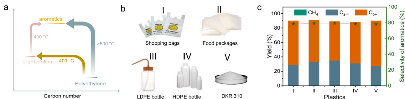
Fig. 5 (a) The temperature for the conversion of various molecules with different enthalpy. (b) Photographs of (I) shopping bags, (II) LDPE bottle, (IV) HDPE bottle, and (V) DKR 310. The component of DKR 310: 92.6% PE and 7.4% impurities (the impurities contain 0.4% Fe powder, 3.7% PS, and 3.3% wood). (c) Data characterizing the aromatization of practical plastics and DKR310 in a dual-bed manner over s -ZSM-5 and Zn/ meso -ZSM-5 catalysts. Reaction conditions: the mixture of 100 mg of practical plastic and 100 mg of s -ZSM-5 in the first bed, 400 mg of Zn/ meso -ZSM-5 for aromatization in the second bed, feed gas of 3.3% H 2 /29.7% Ar/67% N 2 at 3 mL min −1 , 400 °C, 4 h.
