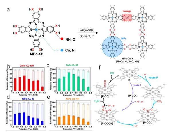
Fig. 25 (a) Synthesis scheme of MPc-Cu-X MOFs. (b-e) FEs of H2 product for different (catalysts). (f) Suggested mechanism for catalytic electrochemical reduction of CO<sub>2</sub> to CO on MPc-Cu-XH MOFs. Reproduced with permission from ref. 236 Copyright 2020, ACS
