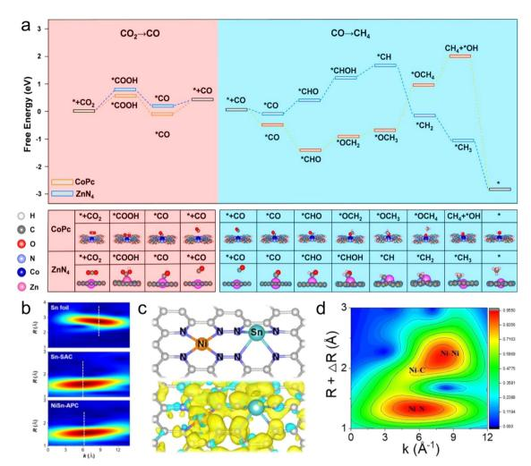
Fig. 29 (a) Free energy profiles and intermediate configuration over CoPc and ZnN $_4$ . Reproduced with permission from ref. 20 Copyright 2020, Wiley. (b) WT analysis of NiSn-APC, Sn-SAC and Sn foil. (c) Spin electron density model proposed for NiSn-APC (yellow; spin up and green; spin down). Reproduced with permission from ref. 261 Copyright 2021, Wiley. (d) WT-EXAFS plot for Ni-CNC-1000. Reproduced with permission from ref. 262 Copyright 2022, Wiley.
