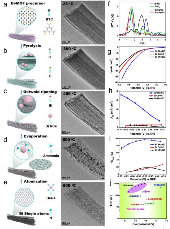
Fig. 23 (a–e) Illustration of the transformation of Bi-MOF to Bi-SA together with corresponding TEM images. (f) EXAFS spectra with  $k^3\chi(k)$  function. (d) LSV curves. (h) Partial current densities of CO. (i) FECO and (j) comparison of TOF values. Reproduced with permission from ref. 212 Copyright 2019, ACS.
