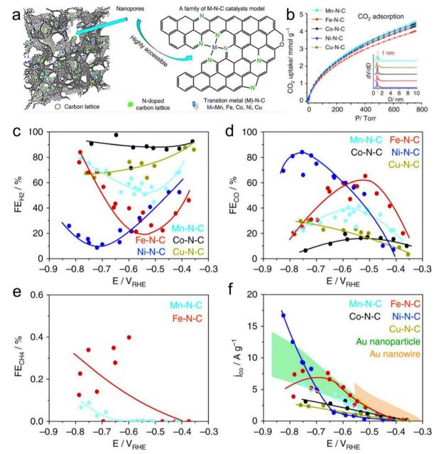
Fig. 17 (a) M-N-C model and structure. (b) Adsorption isotherm curves for  $CO_2$  and inset is the pore size distribution. (c-e) FEs of  $H_2$ , CO and  $CH_4$ , respectively. (f) Mass-normalized partial currents for CO, reproduced with permission from ref. 183 Copyright 2017, Springer Nature.
