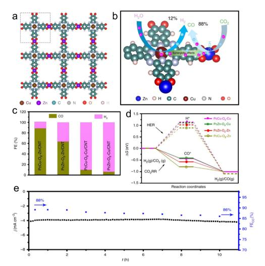
Fig. 19 (a) Illustration of the crystal structure of Zn-PcCu-O<sub>8</sub>. (b) Depiction of CO<sub>2</sub>RR and HER over Zn-PcCu-O<sub>8</sub>. (c) FEs of H<sub>2</sub> and CO for different catalysts. (d) Possible free energy diagram for different catalysts. (e) Amperometry ( $i \sim t$ ) stability test for Zn-PcCu-O<sub>8</sub>/CNT. Reproduced with permission from ref. 189 Copyright 2020, Springer Nature.
