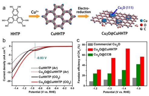
Fig. 9 (a) Design of Cu<sub>2</sub>O@CuHHTP through electrochemical treatment. (b) LSV curves. (c) FE comparison. Reproduced with permission from ref. 151 Copyright 2020, Wiley-VCH.
