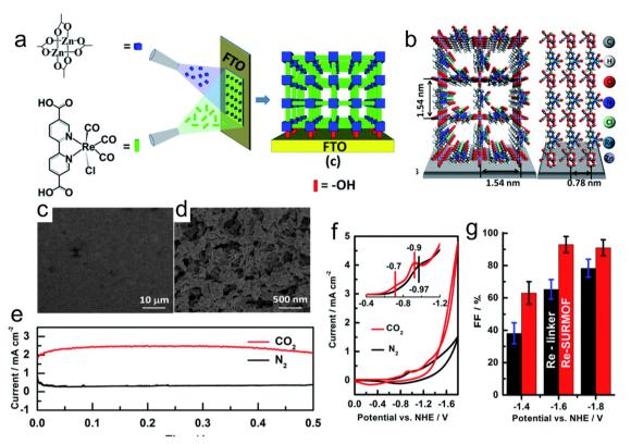
Fig. 13 (a) Schematic synthesis of Re-SURMOF. (b) Crystal structure of Re-SURMOF. (c and d) SEM images of Re-SURMOF. (e) Current density during catalysis of CO<sub>2</sub>RR in CO<sub>2</sub>- and N<sub>2</sub>-saturated electrolyte. (f) Cyclic voltammograms of Re-SURMOF. (g) FE of Re-SURMOF. Reproduced with permission from ref. 165 Copyright 2016, RSC.
