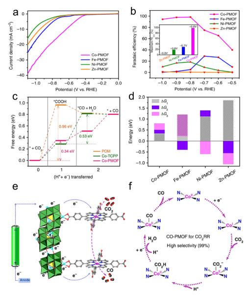
Fig. 14 (a) LSV curves of PMOFs. (b) FEs. (c) Free energy diagram. (d) Free energy comparison of elementary reactions. (e and f) Suggested mechanism for the CO<sub>2</sub>RR on Co-PMOF. Reproduced with permission from ref. 168 Copyright 2018, Springer Nature.
