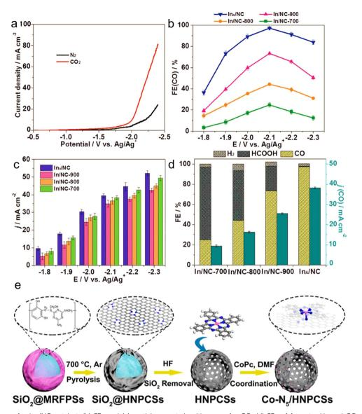
Fig. 26 (a) LSV curves for In<sub>A</sub>/NC catalyst. (b) FEs and (c) partial current densities over for CO. (d) FEs of formate, H<sub>2</sub> and CO. Reproduced with permission from ref. 238 Copyright, 2021 ACS. (e) Schematic of the synthesis of Co-N₅/HNPCSs. Reproduced with permission from ref. 241 Copyright 2018, ACS.
