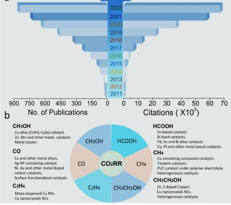
Scheme 2 (a) Trend of publications and citations of electroreduction of carbon dioxide, with data collected from Web of Science. (b) Systematic illustration of metal-based CO<sub>2</sub>RR catalysts and their corresponding products.
