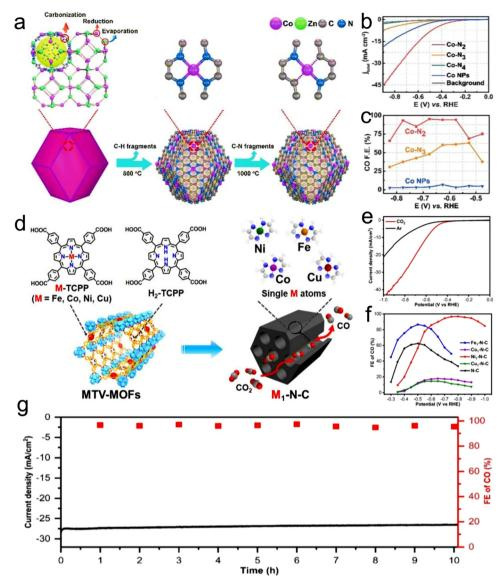
Fig. 16 (a) Co-N<sub>4</sub> synthesis process. (b) LSV curves of all the materials and (c) FEs. Reproduced with permission from ref. 181 Copyright 2021, Wiley. (d) Synthesis of  $M_1-N-C$  single-atom catalysts. (e) LSV curves of  $Ni_1-N-C$ . (f) FEs and (g) durability test of  $Ni_1-N-C$ . Reproduced with permission from ref. 182 Copyright 2020, Wiley-VCH.
