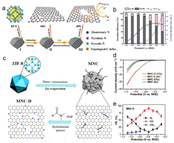
Fig. 21 (a) Synthesis route of defected porous carbon. (b) FEs of CO and H<sub>2</sub> and the partial current densities over DPC. Reproduced with permission from ref. 196 Copyright 2020, Wiley. (c) Synthetic procedure from MNC-D. (d) LSV curves of MNC-D and MNC. (e) FEs over MNC-D. Reproduced with permission from ref. 197 Copyright 2019, Springer.
