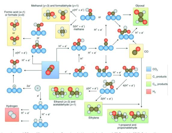
Fig. 5 Reaction pathways of CO<sub>2</sub> to different products. Reproduced with permission from ref. 65 Copyright 2019, Springer Nature.
