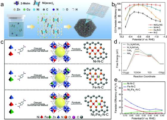
Fig. 24 (a) Schematic description of Ni/Cu-N-C fabrication. (b) FE<sub>CO</sub>. Reproduced with permission from ref. 233 Copyright 2022, ACS. (c) Method for the synthesis of different metal-based catalysts. Reproduced with permission from ref. 234 Copyright 2021, RSC. (d) Free energy diagram for CO<sub>2</sub> conversion. Reproduced with permission from ref. 233 Copyright 2022, ACS. (e) FE of H<sub>2</sub> for various catalysts. Reproduced with permission from ref. 234 Copyright 2021 RSC.
