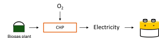
Fig. 1 Schematic representation of combined heat and power (CHP) production: independently from renewable energy availability, biogas is combusted to produce electricity.
