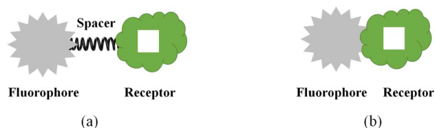
Fig. 3 Fluorescent sensor model (a) with and (b) without a spacer.
