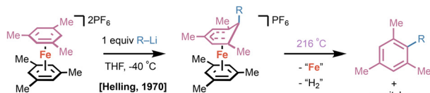
Fig. 1 Helling and coworkers' thermolysis under air to rearomatize and release Fe(II).
