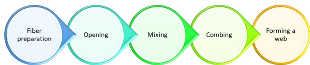
Fig. 3 Steps involved in the formation of nonwovens.
