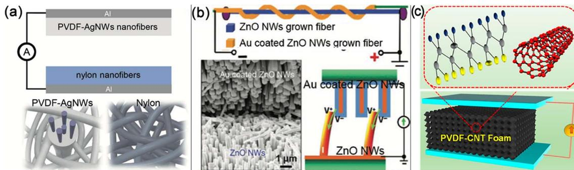
Fig. 1 Schematic diagram for nanogenerators based on 1D materials: (a) PVDF–Ag NW composite and nylon fibers based TENG. Reproduced with permission.<sup>41</sup> Copyright 2017, Wiley. (b) ZnO NW based PENG. Reprinted with permission.<sup>75</sup> Copyright 2008, Springer Nature. (c) Generating piezoelectric charges from a PVDF–CNT foam device. Reprinted with permission.<sup>61</sup> Copyright 2019, Springer Nature.
