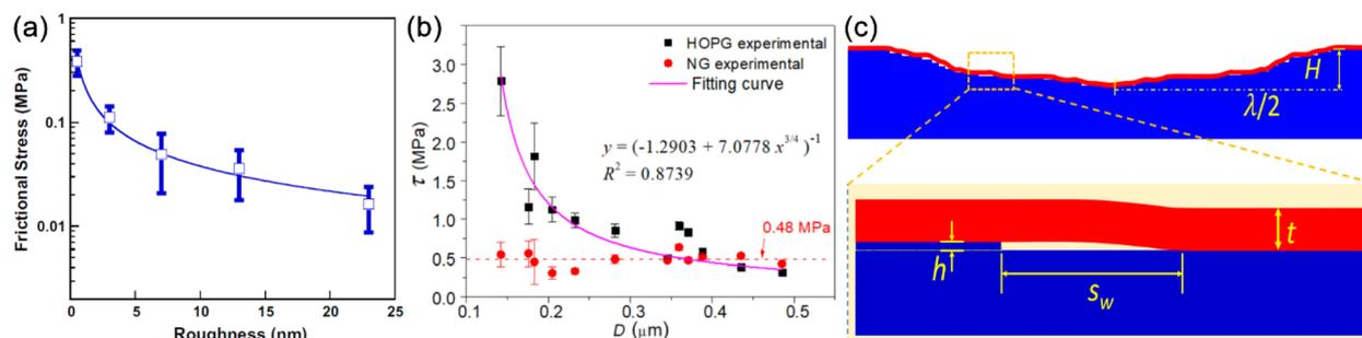
**Fig. 31** (a) Frictional shear stress of SiC NWs against the surface roughness of SiN substrate. Reproduced with permission.<sup>222</sup> Copyright 2017, Springer Nature. (b) Dependences of frictional shear stress of ZnO NWs on HOPG and NG substrates on the NW diameter. (c) Sketches of a NW conforming to a wavy substrate surface and the step-induced gap between the NW and substrate surface. Reproduced with permission.<sup>139</sup> Copyright 2022, Springer Nature.
