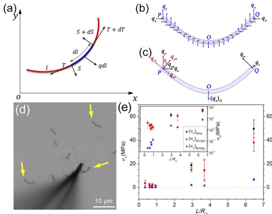
Fig. 22 (a) Schematics of the mechanical model for a bent NW segment held on a substrate by the static friction. (b and c) Distribution of the friction along  $x$  and  $y$  directions. (d) NWs manipulated to the most-bent state by the W tip under OM. (e) Frictional shear stress calculated by different mechanical models versus the  $L/R_O$  value. The inset shows the corresponding values in the logarithmic coordinate. Reproduced with permission.<sup>216</sup> Copyright 2015, IOP.
