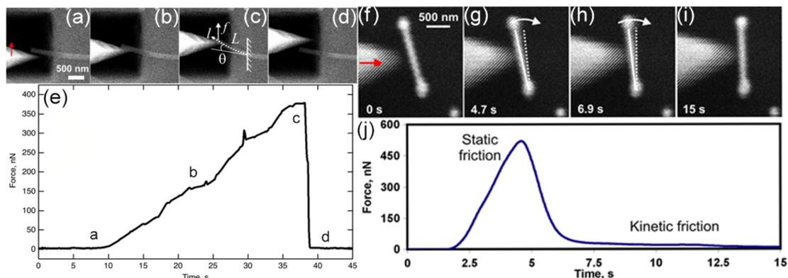
Fig. 17 (a–d) SEM images of the suspended NW being pushed by the tip. (e) The corresponding force curve. Reproduced with permission.<sup>194</sup> Copyright 2011, Elsevier. (f–i) SEM images for the manipulation process of an Ag nanodumbbell. (j) The corresponding recorded tip–nanodumbbell interaction force. Reproduced with permission.<sup>198</sup> Copyright 2015, IOP.
