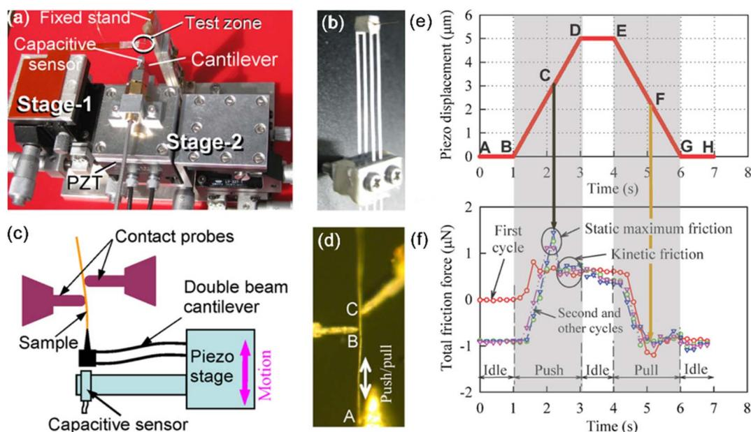
**Fig. 19** (a) Experimental setup for the two-manipulator system. (b) Four-legged parallel beam cantilever. (c) Schematic of friction force measurement system. (d) Optical micrograph of two W probes and the targeted Pt wire. (e) The push–pull cycle of the wire against the probes, corresponding to the piezo displacement during friction measurement, and (f) frictional forces recorded at various cycles. Reproduced with permission.<sup>223</sup> Copyright 2011, Elsevier.
