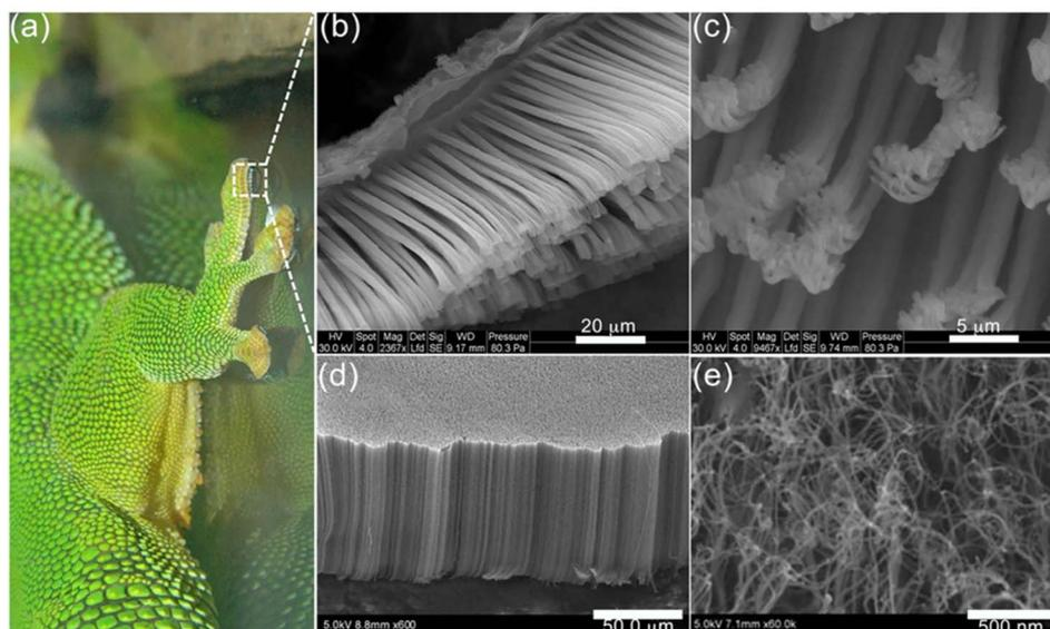
**Fig. 3** (a) Gecko foot attached to a glass substrate, (b) SEM images of setal array, and (c) spatulae at the tip. Reproduced with permission.<sup>103</sup> Copyright 2004, Elsevier. (d) The vertically aligned CNT array and (e) the entangled top layer. Reproduced with permission.<sup>99</sup> Copyright 2008, AAAS.
