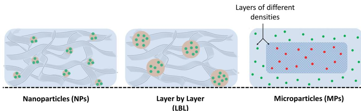
**Fig. 11** Schematic representation of composite systems used to control biomolecule delivery from scaffolds. Nanoparticles (NPs) or microparticles (MPs) embedded within the scaffold matrix as localized biomolecule reservoirs. Layer-by-layer (LBL) assembly, creating stratified layers of varying densities for the precise spatial distribution and controlled release of biomolecules.
