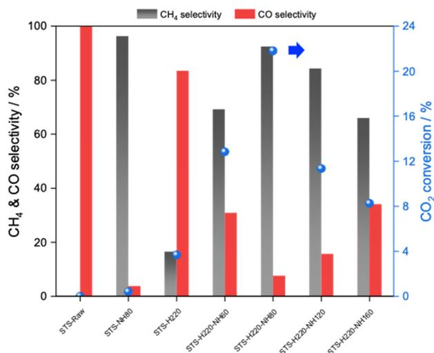
**Fig. 1** CO<sub>2</sub> methanation performance of STS powder samples before and after each treatment step. Reaction conditions:  $T = 300$  °C,  $P = 1$  bar, flow rate = 20 mL min<sup>-1</sup>, reaction gas = H<sub>2</sub>/CO<sub>2</sub>/N<sub>2</sub> = 64/16/20.
