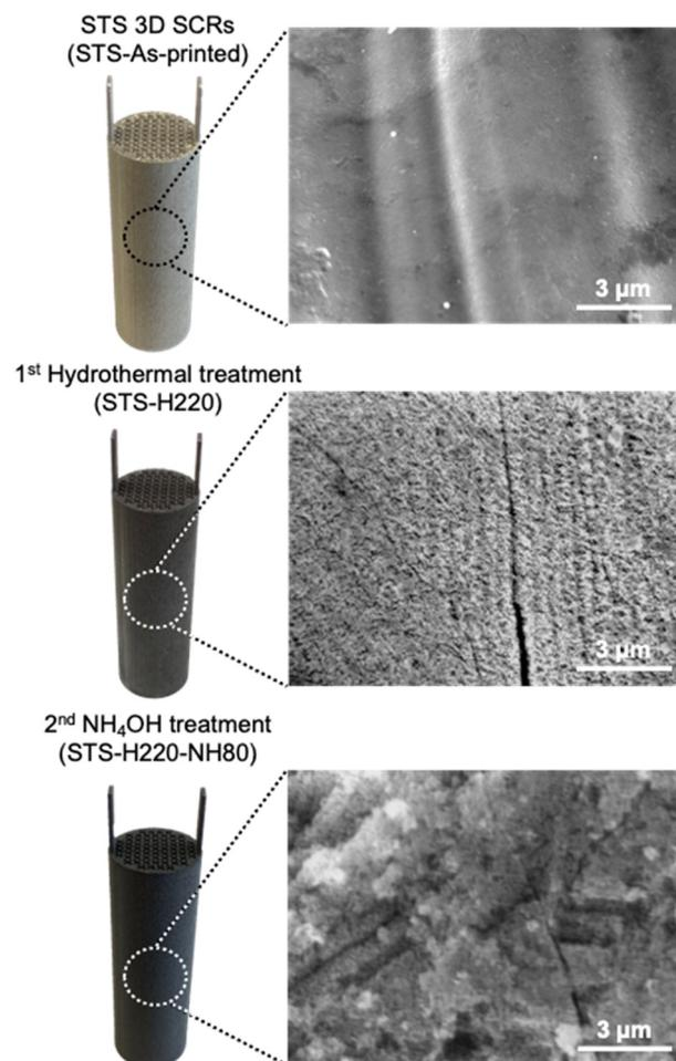
**Fig. 2** Photographs and SEM images of STS 3D SCR before and after each treatment step. The scan speed for the 3D printing process is 1200 mm s<sup>-1</sup>.
