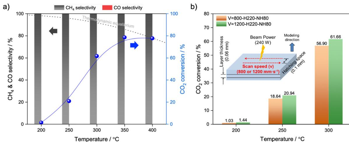
Fig. 4 a) Temperature-dependent  $\text{CO}_2$  conversion with  $\nu = 1200\text{-H220-NH80}$  and b)  $\text{CO}_2$  methanation performance with different scan speeds. Reaction conditions:  $P = 1 \text{ bar}$ , flow rate =  $20 \text{ mL min}^{-1}$ , reaction gas =  $\text{H}_2/\text{CO}_2/\text{N}_2 = 64/16/20$ .
