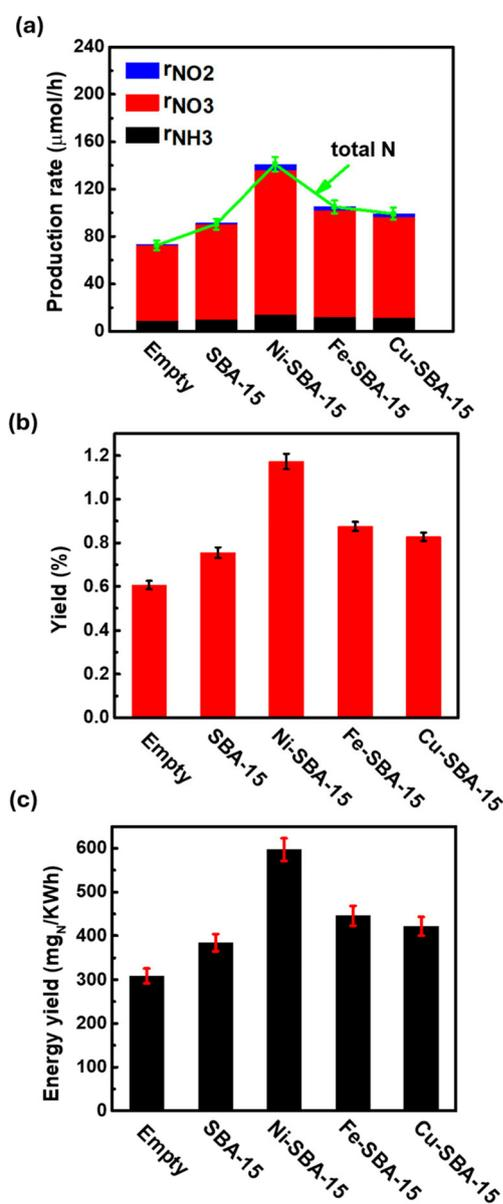
Fig. 10 (a) Production rate of NH<sub>3</sub>, NO<sub>3</sub><sup>-</sup>, and NO<sub>2</sub><sup>-</sup> produced from N<sub>2</sub> and H<sub>2</sub>O with and without catalysts, (b) yield and (c) energy yield of total N obtained from N<sub>2</sub> and H<sub>2</sub>O with and without catalysts, error bars indicate standard deviation [reaction conditions: power of 3.30 W; N<sub>2</sub> flow rate of 40 mL min<sup>-1</sup>, and H<sub>2</sub>O flow rate of 0.1 mL min<sup>-1</sup>].
