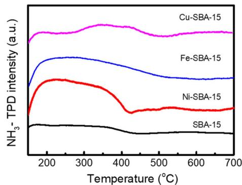
**Fig. 6** NH<sub>3</sub>-TPD spectra of SBA-15, Ni-SBA-15, Fe-SBA-15, and Cu-SBA-15.
