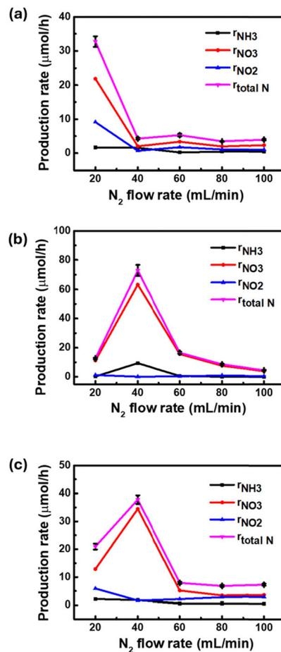
Fig. 9 Nitrogen fixation from  $N_2$  and  $H_2O$ . (a)  $H_2O$  flowrate 0.05  $\text{mL min}^{-1}$ ; (b)  $H_2O$  flowrate 0.10  $\text{mL min}^{-1}$ ; (c)  $H_2O$  flowrate 0.15  $\text{mL min}^{-1}$ , error bars indicate standard deviation.
