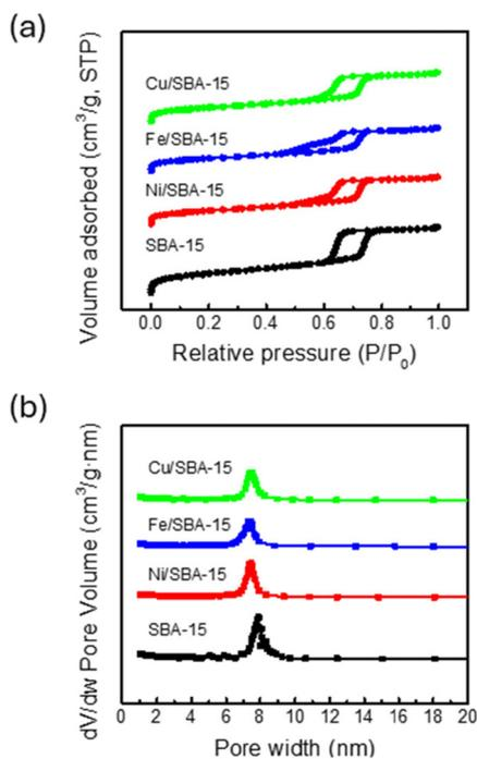
**Fig. 5** N<sub>2</sub> adsorption–desorption isotherms (a) and pore size distributions (b) of SBA-15, Ni-SBA-15, Fe-SBA-15, and Cu-SBA-15.
