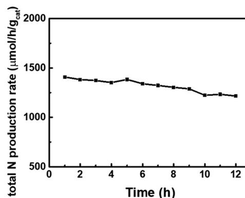
Fig. 11 Stability test of nonthermal plasma-assisted nitrogen fixation from N<sub>2</sub> and H<sub>2</sub>O over the Ni-SBA-15 catalyst [reaction conditions: power of 3.30 W; N<sub>2</sub> flow rate of 40 mL min<sup>-1</sup>, and H<sub>2</sub>O flow rate of 0.1 mL min<sup>-1</sup>].
