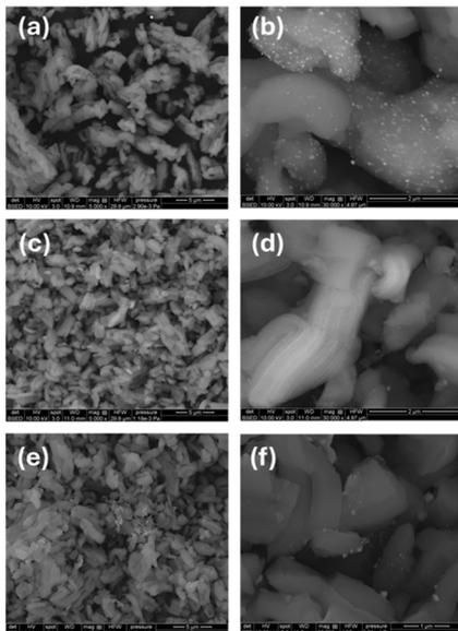
Fig. 3 SEM images of Ni-SBA-15 (a and b), Fe-SBA-15 (c and d), and Cu-SBA-15 (e and f).
