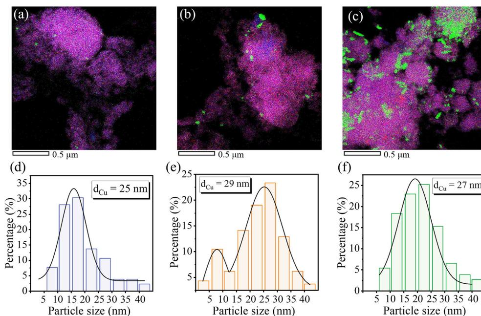
**Fig. 5** Morphological characterisation. (a)–(c) EDX maps of selected areas from 1\_STO, 2\_STO, and 5\_STO post H<sub>2</sub>-TPR with associated (d)–(f) particle size distribution. Note: green areas in (a–c) represent counts from copper species on the Ti + Sr + O overlay given in purple.
