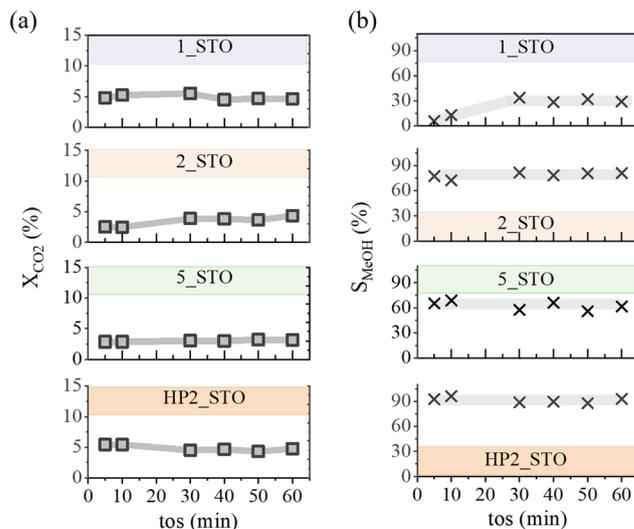
Fig. 1 Flow test response. Time on stream (tos, min) profiles of (a) carbon dioxide conversion ( $X_{CO_2}$ , %) and (b) methanol selectivity ( $S_{MeOH}$ , %) over (from top to bottom) 1\_STO, 2\_STO, 5\_STO and HP2\_STO catalysts, respectively. Reaction conditions:  $P = 30$  bar,  $T = 200$  °C, GHSV = 26 000 h<sup>-1</sup>.
