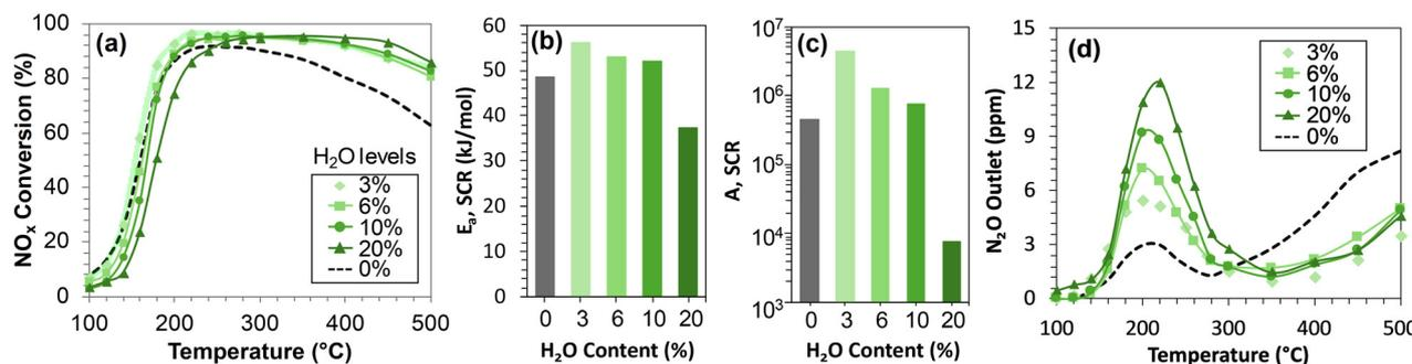
Fig. 1 (a) Steady state standard SCR NO<sub>x</sub> conversion at different feed H<sub>2</sub>O content (0, 3, 6, 10, 20%) on Cu-SSZ-13, (b) SCR activation energy, (c) SCR pre-exponential factor, (d) N<sub>2</sub>O byproduct formation during SCR.
