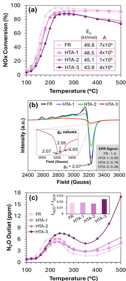
**Fig. 3** (a) SCR NO<sub>x</sub> conversion on four Cu-SSZ-13 samples with varied aging treatment: FR, HTA-1, HTA-2, HTA-3. (b) X-band EPR spectra of FR, HTA-1, HTA-2 and HTA-3 samples. Insets show ratios of total EPR signal relative to FR and high field region of HTA-3. (c) N<sub>2</sub>O byproduct formation during SCR.
