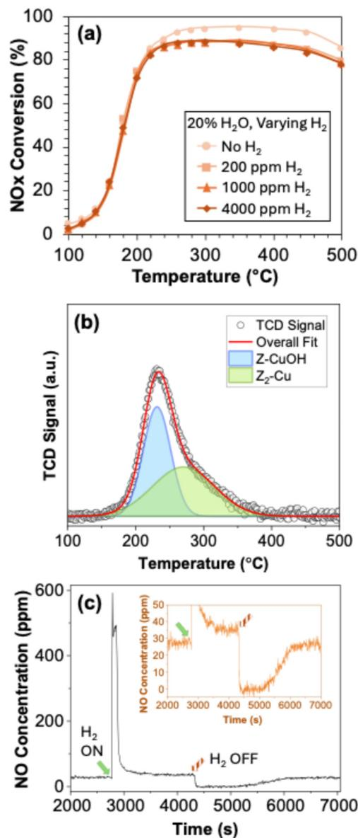
Fig. 2 (a) Steady-state SCR NO<sub>x</sub> conversion under 0, 200 ppm, 1000 ppm, and 4000 ppm H<sub>2</sub>, (b) H<sub>2</sub>-TPR of Cu-SSZ-13, (c) NO transient during SCR at 250 °C with and without 200 ppm H<sub>2</sub>.
