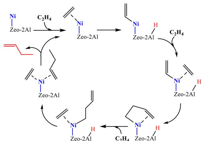
**Scheme 9** Proposed Cossee-Arlman pathway for ethylene dimerization to 1-butene on isolated  $\text{Ni}^{2+}$ ; Zeo = Ni-FAU zeolite. This scheme has been adapted from ref. 30 with permission from Wiley-VCH GmbH, copyright 2025.
