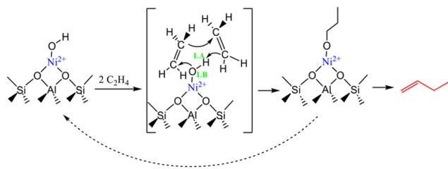
**Scheme 12** Probable ethene dimerization catalytic cycle on  $(\text{Ni-OH})^+$  moieties acting as a Lewis acid-base pair proposed from a DFT analysis of ethene reactions on Ni-Al-MCM-41. This scheme has been adapted from ref. 51 with permission from American Chemical Society, copyright 2025.
