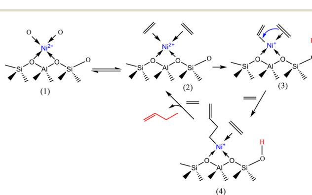
**Scheme 8** Proposed mechanism for the dimerization of ethylene by Ni-AIKIT-6. (1) Nickel complexation; (2) ethylene complexation; (3) metal–vinyl intermediate; (4) 1-butene formation. This scheme has been adapted from ref. 46.
