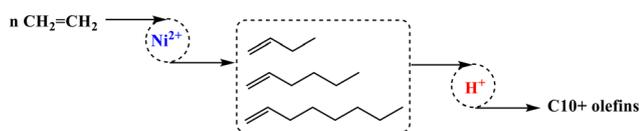
**Scheme 15** Main reaction pathways of ethylene oligomerization into C<sub>10+</sub> olefins by catalytic cascade reactions.
