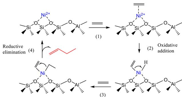
**Scheme 6** Simplified catalytic cycle proposed for the activation and dimerization of ethylene on the active  $\text{Ni}^{2+}$  centers of Ni-Beta catalysts: (1) ethylene adsorption on Ni site; (2) oxidative addition; (3) ethylene insertion; (4) reductive elimination of butene. This scheme has been adapted from ref. 7 with permission from American Chemical Society, copyright 2025.
