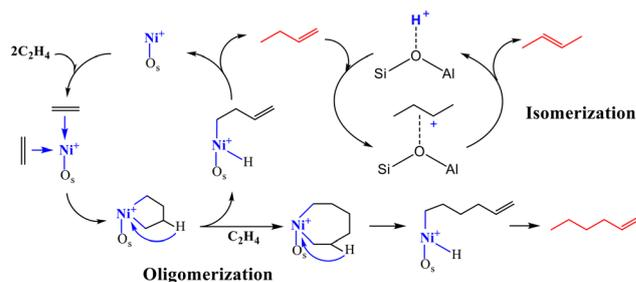
**Scheme 11** Proposed catalytic cycles for linear ethylene oligomerization involving  $\text{Ni}^+$  and  $\text{H}^+$  as active sites on the Ni-AlSBA-15 catalyst ( $\text{O}_s^{2-}$  = surface oxide ions). This scheme has been adapted from ref. 40.
