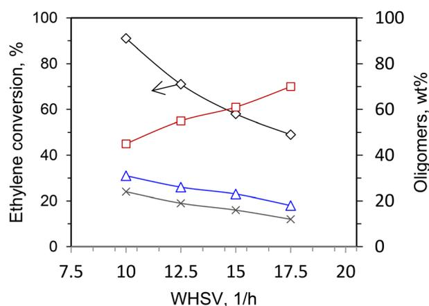
Fig. 5 Ethylene conversion and oligomer distribution at various WHSV; Ni-SBA-15 catalyst; (○) % ethylene conversion, (□) % C<sub>4</sub>, (Δ) % C<sub>6</sub>, (x) C<sub>8+</sub>; conditions: 3.0 MPa of ethylene, T = 150 °C, TOS = 1 h. This scheme has been reproduced from ref. 40.
