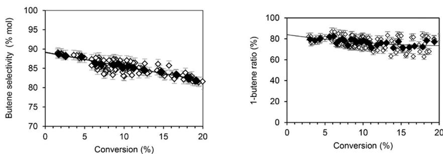
**Fig. 3** Butene selectivity (left) and 1-C4 isomer ratio (right) vs. ethylene conversion. Catalyst: 0.1 g of Ni-AIKIT-6,  $T = 40\text{--}80\text{ }^{\circ}\text{C}$ ,  $P_{\text{ethylene}} = 0.4\text{--}2\text{ MPa}$ ,  $P_{\text{total}} = 3.0\text{ MPa}$ , contact time = 15–98 s. This scheme has been reproduced from ref. 46.
