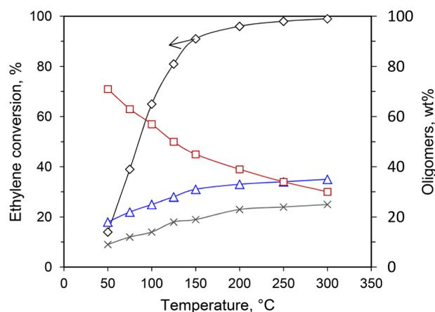
Fig. 4 Ethylene conversion and oligomer distribution at various temperatures; Ni-SBA-15 catalyst; (◇) % ethylene conversion, (□) % C<sub>4</sub>, (Δ) % C<sub>6</sub>, (x) C<sub>8</sub>; conditions: 3.0 MPa, WHSV = 10 h<sup>-1</sup>. This scheme has been reproduced from ref. 40.
