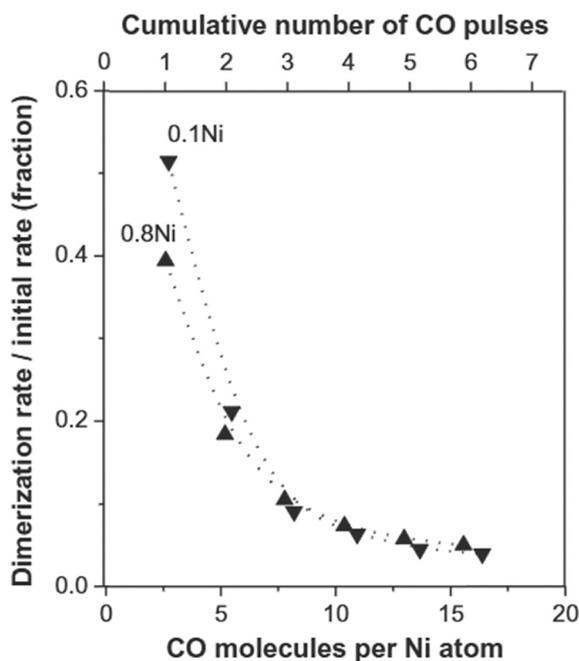
Fig. 6 Ratio of rates after each CO pulse introduction (per Ni) at  $-30\text{ }^\circ\text{C}$ , 1.5 MPa ethene. This figure has been reproduced from ref. 52 with permission from Elsevier, copyright 2025.
