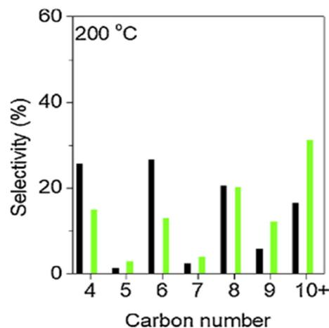
**Fig. 15** Carbon distribution of products obtained after ethylene reaction for 16 h on stream over Ni/Siral-30 (black) and Ni/Siral-30 + H-ZSM-5 (green) in the continuous fixed-bed reactor. This figure has been reproduced from ref. 75 with permission from Elsevier, copyright 2025.
