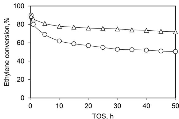
Fig. 10 Ethylene conversion vs. time on stream in the presence of (○) C<sub>2</sub>H<sub>4</sub> + N<sub>2</sub> and (Δ) C<sub>2</sub>H<sub>4</sub> + N<sub>2</sub> + H<sub>2</sub> over the Ni-ASA catalyst. Reaction conditions: T = 250 °C, P = 1.5 MPa, WHSV = 1.1 h<sup>-1</sup>. This scheme has been reproduced from ref. 39.
