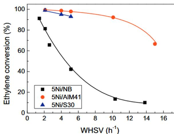
Fig. 9 Ethylene conversion over Ni-Beta (5Ni/NB), Ni-MCM-41 (5Ni/AlM41) and Ni-ASA (5Ni/S30) catalysts. Reaction conditions: T = 120 °C, P<sub>tot</sub> = 3.5 MPa, P<sub>C<sub>2</sub></sub> = 2.6 MPa. This figure has been reproduced from ref. 12 with permission from Elsevier, copyright 2025.
