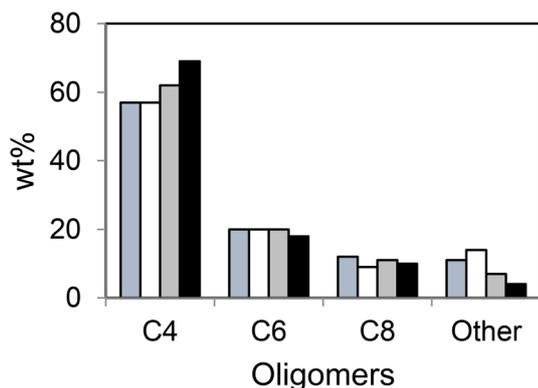
Fig. 8 Effect of the contaminants on the product distribution; blue = C<sub>2</sub>H<sub>4</sub> + N<sub>2</sub>, white = C<sub>2</sub>H<sub>4</sub> + N<sub>2</sub> + H<sub>2</sub>, grey = C<sub>2</sub>H<sub>2</sub> + N<sub>2</sub> + CO, black = C<sub>2</sub>H<sub>2</sub> + N<sub>2</sub> + H<sub>2</sub>O; TOS = 30 h, T = 250 °C, catalyst: Ni-ALSBA-15. This scheme has been reproduced from ref. 39.
