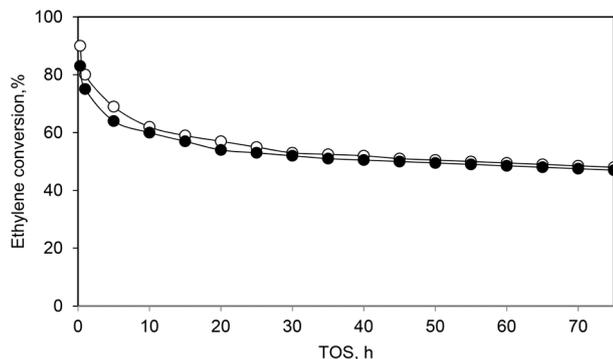
Fig. 12 Ethylene conversion vs. time on stream, over (○) fresh and (●) regenerated Ni-ALSiO<sub>2</sub> catalyst; reaction conditions: C<sub>2</sub>H<sub>4</sub>/N<sub>2</sub> = 1/5 (vol), T = 250 °C, P = 15 bar, WHSV = 1.1 h<sup>-1</sup>. This scheme has been reproduced from ref. 39.
