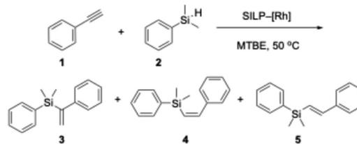
**Scheme 2** Biphasic, continuous-flow hydrosilylation between PA (**1**) and DMPS (**2**) with **Rh-1** in the SILP formed by [BMIM][BF<sub>4</sub>] on a macro-mesoporous silica monolith. Stationary phase: solid silica and SILP (containing **Rh-1**), mobile phase: MTBE (containing reactants and products).
