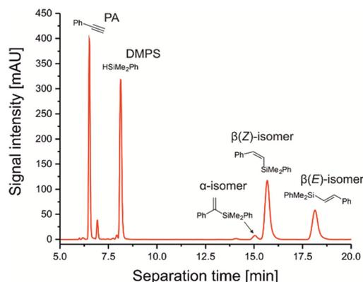
**Fig. 4** Chromatogram of the reaction solution, recorded by UV/vis diode-array detection at 260 nm, highlighting the baseline separation of compounds 1-5. Column: 3.0 mm inner diameter  $\times$  100 mm length packed with phenyl-hexyl-modified, fully porous silica particles (1.8  $\mu\text{m}$  particle size, 9.5 nm mesopore size), mobile phase: 75/25 (v/v) methanol/water, flow rate:  $0.6 \text{ mL min}^{-1}$ , column backpressure: 800 bar.
