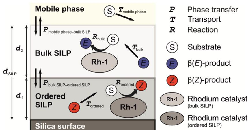
**Fig. 10** Schematic representation of relevant structural and dynamic aspects in the continuous-flow hydrosilylation reaction between PA and DMPS with Rh-1 in the SILP formed by [BMIM][BF<sub>4</sub>] in the ~30 nm wide mesopores of a (macro-mesoporous) silica monolith.
