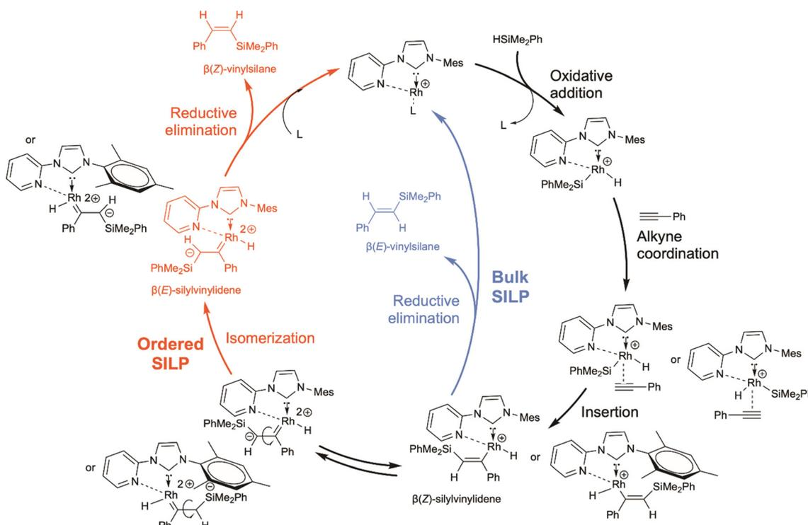
**Scheme 3** Modified Chalk-Harrod mechanism for the preferential formation of  $\beta(Z)$ - or  $\beta(E)$ -vinylsilane isomer in the continuous-flow hydrosilylation reaction between PA and DMPS with Rh-1 in the SILP formed by [BMIM][BF<sub>4</sub>] on a macro-mesoporous silica monolith.
