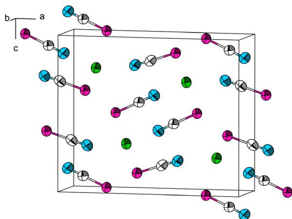
Fig. 8 The crystal structure of Pb[SeCN]<sub>2</sub>. Thermal ellipsoids are drawn at the 90% probability level at 100 K. Green: Pb, white: C, blue: N, magenta: Se.
