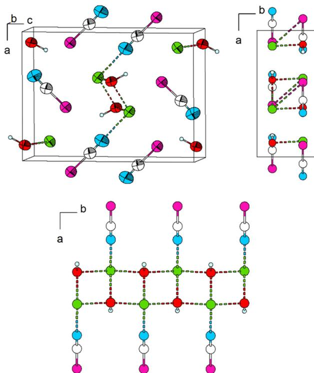
**Fig. 13** The crystal structure of  $\text{Pb}[\text{SeCN}][\text{OH}]$ . Top left: view of the unit cell approximately along  $[010]$ . Top right: view of the unit cell along  $[001]$ . Bottom: double-chain of Pb–[OH] units, which runs along  $[010]$ . Green: Pb, white: C, blue: N, magenta: Se, red: O, light blue: H. Thermal ellipsoids are drawn at the 90% probability level at 180 K, and hydrogen atoms are drawn with an arbitrary radius.
