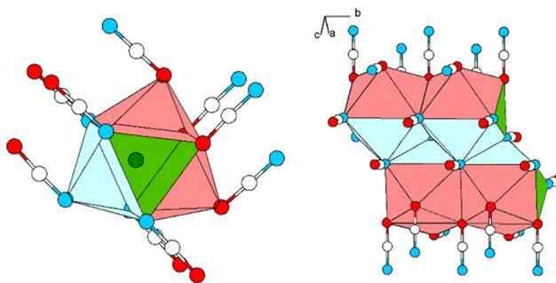
**Fig. 2** Excerpt of the crystal structure of  $\text{Pb}[\text{OCN}]_2$ . Left: coordination polyhedron around Pb. Right: double-chain of polyhedra around Pb extending along  $[010]$ . Green: Pb, white: C, blue: N, red: O.
