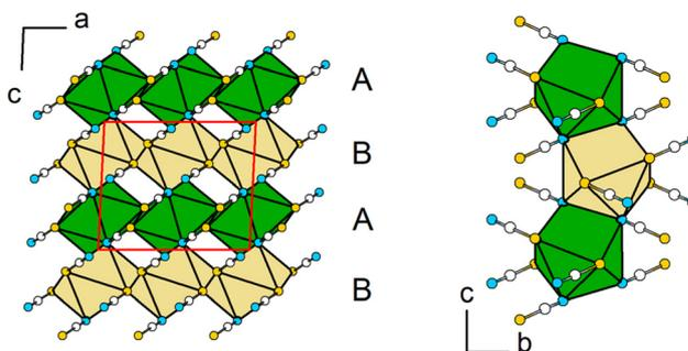
**Fig. 7** Extended crystal structure views of  $\text{Pb}[\text{SCN}]_2$  emphasizing the stacking of the coordination polyhedra around Pb. Left: view along  $[010]$  with layers of antiprisms around Pb atoms forming an ABAB motif stack along  $[001]$ . Right: view along  $[100]$ , emphasizing the common  $N,N$ -edges of the polyhedra. Green: Pb, white: C, blue: N, yellow: S.
