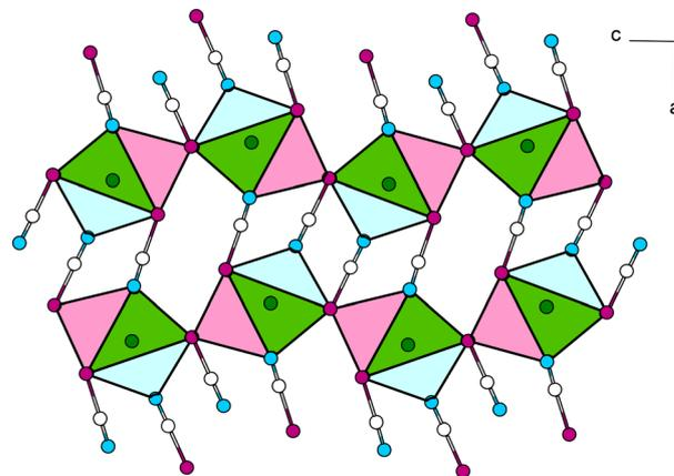
Fig. 10 View of the crystal structure of Pb[SeCN]<sub>2</sub> along [010]. Coordination polyhedra around Pb atoms are connected *via* common [SeCN]<sup>−</sup> units. Green: Pb, white: C, blue: N, magenta: Se.
