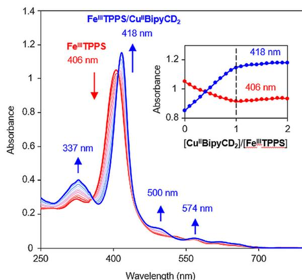
**Fig. 4** UV-visible titration of  $\text{Fe}^{\text{III}}\text{TPPS}$  (10  $\mu\text{M}$ ) in 0.05 M phosphate buffer with the stepwise addition of  $\text{Cu}^{\text{II}}\text{BipyCD}_2$  in water. The inset shows changes in absorbance as a function of ratio of the concentrations  $[\text{Cu}^{\text{II}}\text{BipyCD}_2]/[\text{Fe}^{\text{III}}\text{TPPS}]$ .
