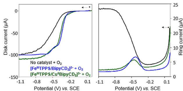
**Fig. 9** Voltammograms measured by RRDE experiments of the various complexes (10 μL of a 2.5 mM solution) coated with Nafion (10 μL) on the disk electrode in O<sub>2</sub>-saturated solution, measured at pH 7 in 0.05 M phosphate buffer containing 0.5 M Na<sub>2</sub>SO<sub>4</sub> at a scan rate of 0.02 V s<sup>-1</sup> and 100 rpm.
