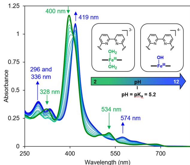
**Fig. 3** UV-visible spectral changes of  $\text{Fe}^{\text{III}}\text{TPPS}/\text{BipyCD}_2$  (10  $\mu\text{M}$ ) in aqueous 0.1 M  $\text{NaClO}_4$  as a function of the pH of the solution from 2 to 12. The pH was adjusted by addition  $\text{HClO}_4$  and  $\text{NaOH}$ .
