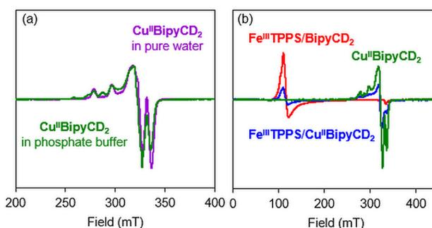
Fig. 6 EPR spectra at 25 K of (a)  $[\text{Cu}^{\text{II}}\text{BipyCD}_2]^{2+}$  ( $0.5 \mu\text{M}$ ) in water (purple line) or in  $0.025 \mu\text{M}$  phosphate buffer at pH 7 (green line) and (b)  $[\text{Fe}^{\text{III}}\text{TPPS}/\text{BipyCD}_2]^{3-}$  (red line),  $[\text{Cu}^{\text{II}}\text{BipyCD}_2]^{2+}$  (green line) and  $[\text{Fe}^{\text{III}}\text{TPPS}/\text{Cu}^{\text{II}}\text{BipyCD}_2]^{2-}$  (blue line) in  $0.025 \text{ M}$  phosphate buffer at pH 7.
