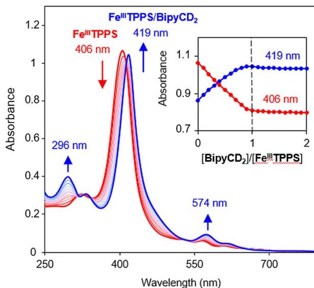
Fig. 2 UV-visible titration of **Fe<sup>III</sup>TPPS** (10  $\mu$ M) in 0.05 M phosphate buffer with the stepwise addition of **BipyCD<sub>2</sub>** in phosphate buffer. The inset shows changes in absorbance as a function of [**BipyCD<sub>2</sub>**]/[**Fe<sup>III</sup>TPPS**] concentrations.
