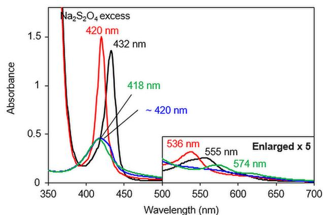
**Fig. 8** UV-visible spectra of 6 μM solutions of the [Fe<sup>III</sup>TPPS/Cu<sup>I</sup>BipyCD<sub>2</sub>]<sup>-</sup> complex (green line), its reduced Fe<sup>II</sup>/Cu<sup>I</sup> (black line), oxygenated Fe<sup>III</sup>-O<sub>2</sub><sup>-</sup>/Cu<sup>I</sup> (blue line) and carbonylated Fe<sup>II</sup>-CO/Cu<sup>I</sup> (red line) products in 0.05 M phosphate buffer at pH 7. The inset shows an enlargement of the Q-band region.
