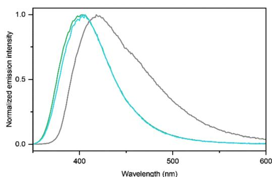
**Fig. 4** Photoluminescence emission spectra for Si(O<sup>1</sup>NO<sup>2</sup>)<sub>2</sub> as crystal-line powder (grey trace), 10 wt% doped thin film in PMMA (green trace) and 10 wt% doped thin film in PS (aqua trace). Spectra were recorded upon excitation at  $\lambda_{\text{exc}} = 320$  nm.
