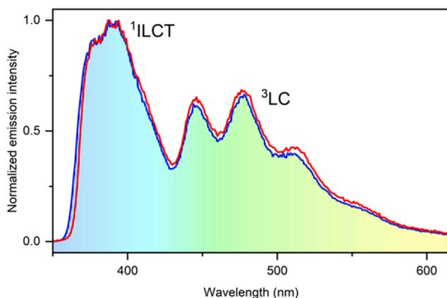
**Fig. 5** Low-temperature photoluminescence emission spectra in a toluene glassy matrix at 77 K of  $\bar{A}$ - $\text{Si}(\text{O}^1\text{NO}^2)_2$  (first eluted, blue trace) and  $\Delta$ - $\text{Si}(\text{O}^1\text{NO}^2)_2$  (second eluted, red trace). Spectra were recorded upon excitation at  $\lambda_{\text{exc}} = 320$  nm.
