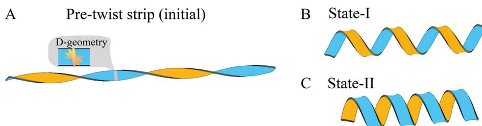
**Fig. 12** Deformations of an LCE strip with pre-twist. (A) The initial twisted shape with the D-geometry. We obtain (B) state-I after  $T$  decreases from  $T/T_{NI} = 0.96$  to  $T/T_{NI} = 0.85$  and (C) state-II after  $T$  increases from  $T/T_{NI} = 0.96$  to  $T/T_{NI} = 1.05$ .
