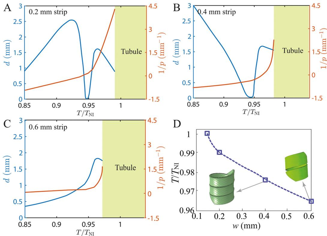
Fig. 10 Varying strip width  $w$  in strips with prebend along the  $\Psi = 45^\circ$  axis. Temperature dependence of  $d$  and  $p$  for a 0.2 mm strip (A), a 0.4 mm strip (B) and a 0.6 mm strip (C). (D) Normalized formation temperature of the tubule shape as a function of strip width.
