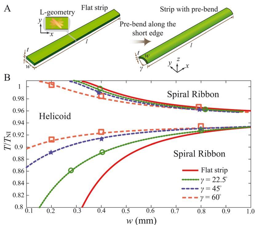
Fig. 4 Pre-bend along the short axis facilitates a spiral ribbon shape for a narrow strip. (A) Schematics of a strip with pre-bend along its short axis. (B) State diagram for a flat strip and three pre-bend strips (along the short axis at different angles) with  $w = 0.2$  mm.
