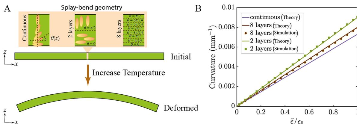
**Fig. 1** A flat LCE strip with a continuous and step-wise splay-bend director field. (A) Schematics of the deformation of a strip with splay-bend alignment. (B) A comparison of our simulations and theories.<sup>41</sup>
