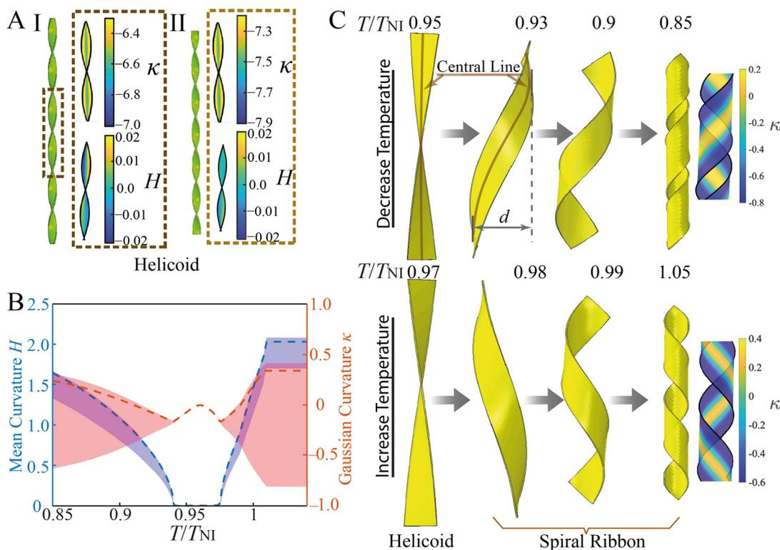
**Fig. 3** Characterization of helicoids and spiral ribbons formed from flat strips. (A) A narrow L-geometry strip ( $w = 0.2$  mm): Gaussian curvature  $\kappa$  and mean curvature  $H$  for the helicoid shape at state-I ( $T/T_{\text{NI}} = 0.85$ ) and state-II ( $T/T_{\text{NI}} = 1.05$ ). (B) Temperature dependence of  $H$  and  $\kappa$  of a wide strip with  $w = 0.76$  mm. (C) Snapshots during the deformation of a wide strip ( $w = 0.76$  mm).
