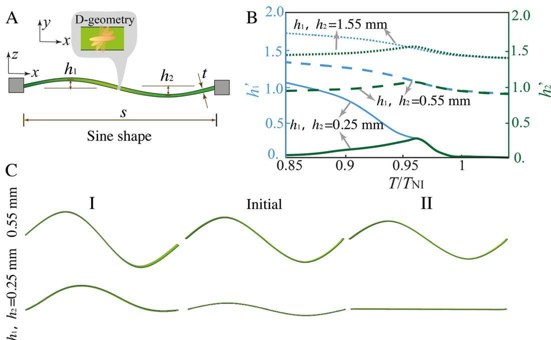
**Fig. 13** Deformations of a constrained LCE strip in sinusoidal shape. (A) Schematics of a constrained strip in the sinusoidal shape. (B) Temperature dependence of parameters  $h_1'$  and  $h_2'$ . (C) Snapshots at state-I ( $T/T_{NI} = 0.85$ ), the initial state ( $T/T_{NI} = 0.96$ ), and state-II ( $T/T_{NI} = 1.05$ ) for two constrained sinusoidal strips.
