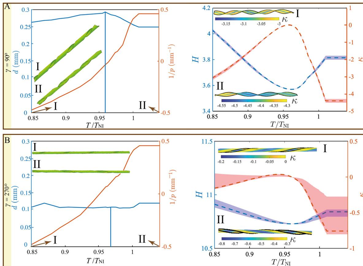
**Fig. 6** The deformations of 0.2 mm strips with larger pre-bend angles along the short axis. (A)  $\gamma = 90^\circ$ . (B)  $\gamma = 270^\circ$ . State-I is for  $T/T_{NI} = 0.85$  and state-II is for  $T/T_{NI} = 1.05$ .
