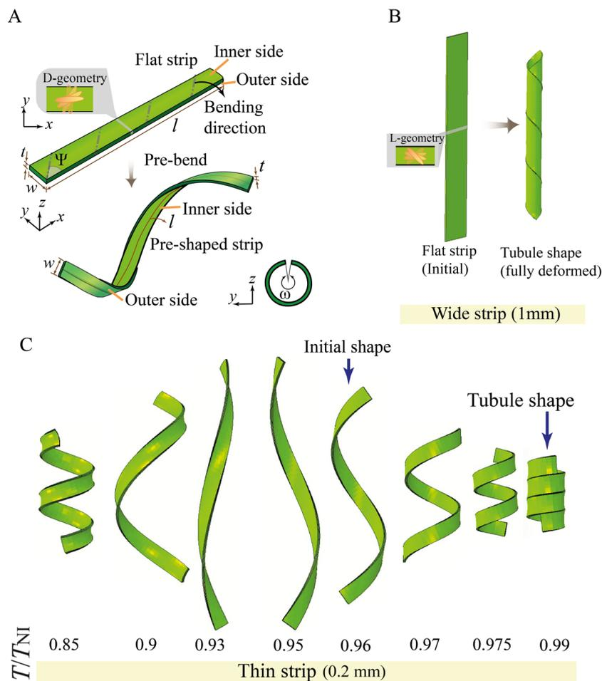
**Fig. 9** Pre-bend along the  $\Psi = 45^\circ$  axis. (A) Schematics of a strip pre-bending into a helical shape. (B) A tubule from a wide flat strip with  $w = 1$  mm. (C) A tubule shape from a narrow pre-shaped strip with  $w = 0.2$  mm.
