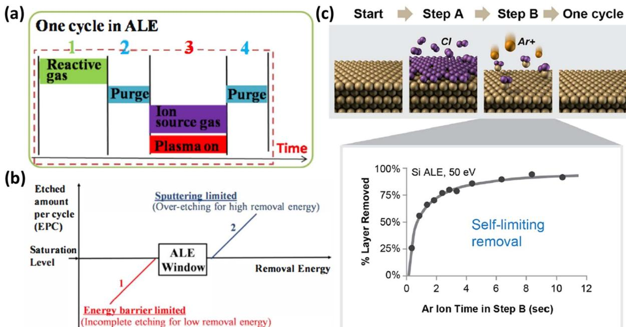
Fig. 4 (a) One cycle in the ALE process. (b) Etched amount per cycle (EPC) vs. removal energy. (c) Schematic of ALE steps and self-limiting removal.<sup>38</sup>
