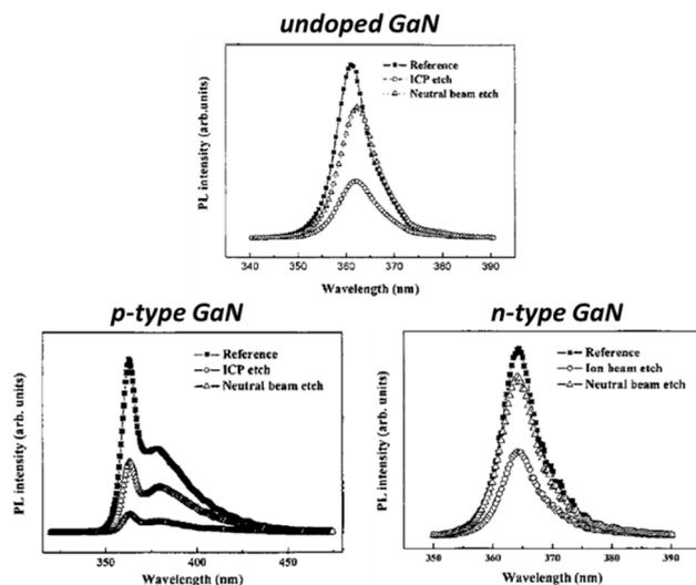
Fig. 11 PL data of undoped GaN, p-type GaN, and n-type GaN after etching with ICP and neutral beams, with the reference samples being unetched.<sup>55</sup>
