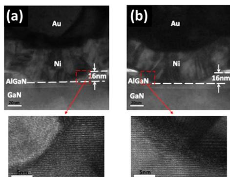
Fig. 12 HRTEM of the gate recess AlGaIn etching region and zoom-in images (a) by neutral beam etching (b) by ICP-RIE.<sup>58</sup>
