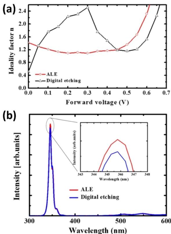
Fig. 8 (a) Photoluminescence intensity comparison between ALE and digital etching. (b) Ideality factor behavior in the forward voltage range.<sup>53</sup>
