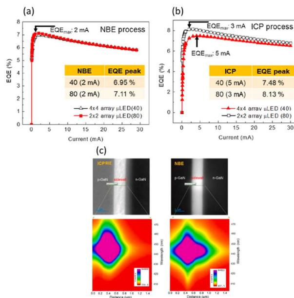
Fig. 13 EQE of micro-LED arrays processed by (a) NBE and (b) ICP-RIE. (c) CL analysis in the blue-light wavelength region: NBE vs. ICP-RIE.<sup>65,66</sup>
