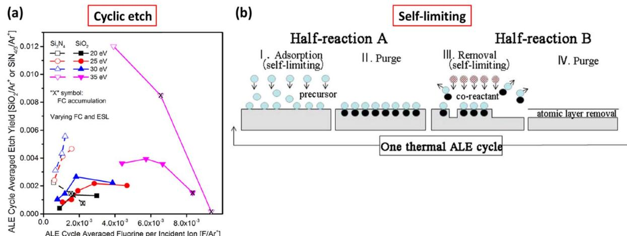
Fig. 5 Two fundamental aspects of ALE: (a) cyclic Etch<sup>40</sup> and (b) self-limited etching.<sup>41</sup>
