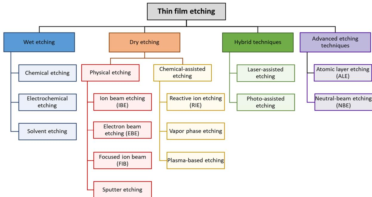
Fig. 2 Classification of thin film etching techniques.
