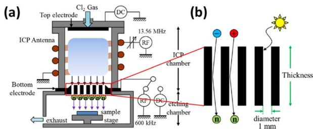
Fig. 9 (a) Neutral beam etching system. (b) Carbon aperture array.<sup>54</sup>
