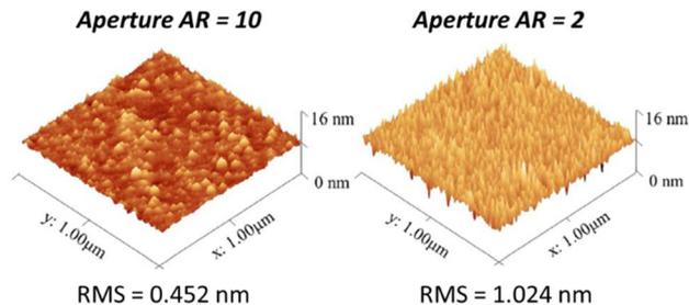
Fig. 10 AFM images of the AlGaIn surface with different carbon aperture aspect ratio designs.<sup>64</sup>
