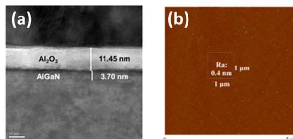
**Fig. 7** MIS-HEMT with a recessed gate structure. (a) TEM cross-section image in the gate recess region, highlighting a smoothly etched surface and precise etching control. (b) Surface morphology of the recessed gate region, revealing a surface roughness ( $R_a$ ) of 0.4 nm, as inspected by AFM.<sup>47</sup>
