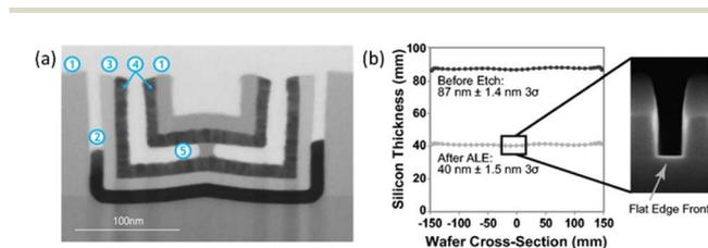
**Fig. 6** (a) Example of etch selectivity in thermal ALE at 250 °C. Materials are (1) SiN, (2) HfO<sub>2</sub>, (3) SiO<sub>2</sub>, (4) TiN, and (5) Al<sub>2</sub>O<sub>3</sub>. No measurable removal in SiN, SiO<sub>2</sub>, and TiN was detected after 1000 ALE cycles.<sup>46</sup> (b) Plasma-assisted ALE results showing characteristic ALE benefits with excellent depth uniformity across the wafer and flat silicon etch front on the feature.<sup>26</sup>
