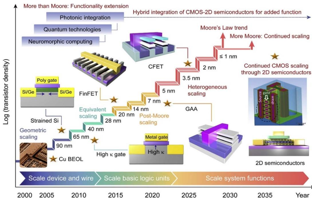
Fig. 1 Evolution of transistor density and gate length in ICs.<sup>1</sup>
