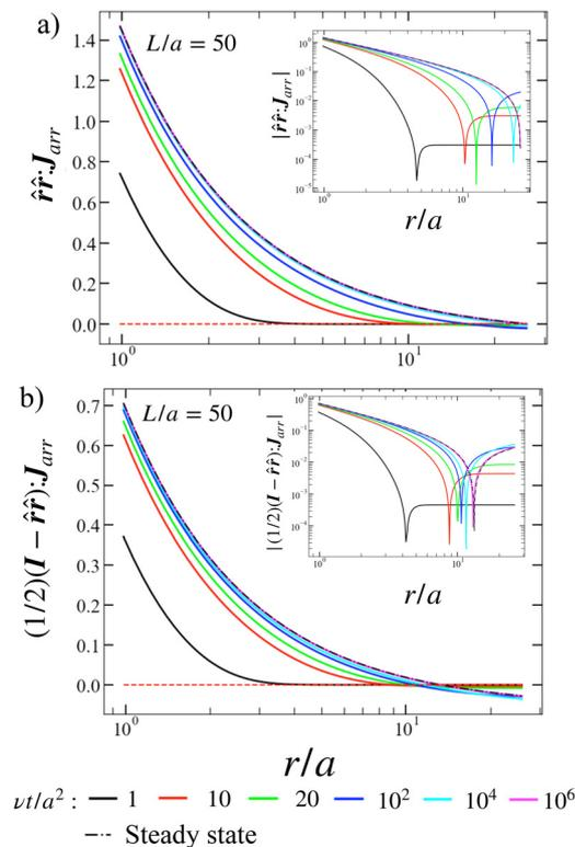
**Fig. 4** Projections of the start-up flow Green's function (a) along and (b) perpendicular to a test particle in a periodic array. The array has simple cubic cell symmetry and a unit cell size  $L/a = 50$ . Due to the spherical symmetry of eqn (31), these two components are sufficient to specify the tensor.
