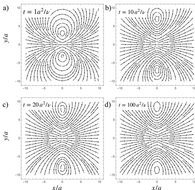
**Fig. 2** Streamlines for the velocity field of a test particle located at the origin and part of a periodic array with simple cubic symmetry and a unit cell size  $L/a = 50.$  The external force is applied at  $t = 0$  and points in the positive  $x$ -direction. The plots (a), (b), (c), and (d) correspond to times  $ta^2/\nu = 1, 10, 20,$  and  $100,$  respectively, after the force is applied.
