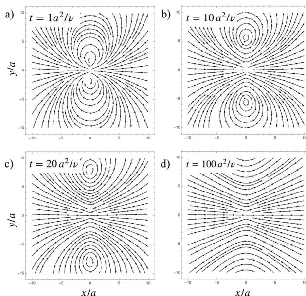
**Fig. 1** Streamlines for the velocity field of an isolated particle at the origin. The external force is applied at  $t = 0$  and points in the positive  $x$ -direction. The plots (a), (b), (c), and (d) correspond to times  $ta^2/\nu = 1, 10, 20,$  and  $100,$  respectively, after the force is applied.
